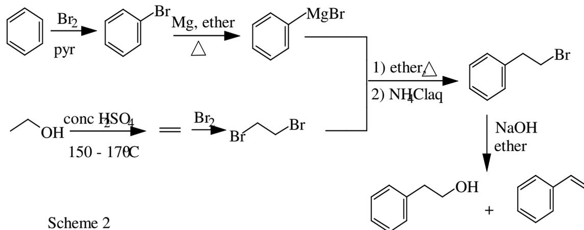
**Scheme 2.** Synthetic pathway to 2-phenylethanol.
