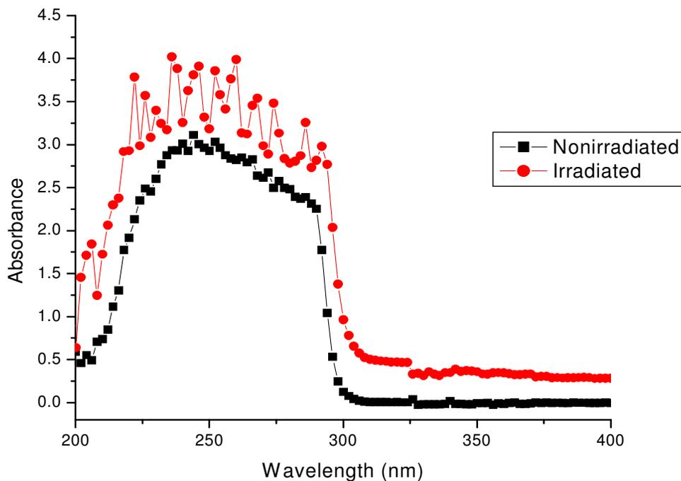
**Figure 2.** Variation in the absorbance values of the irradiated and nonirradiated films (60 phr).
