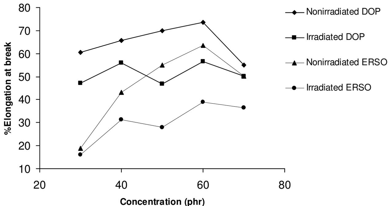
Figure 4. Variation in elongation at break with plasticizer concentration.
