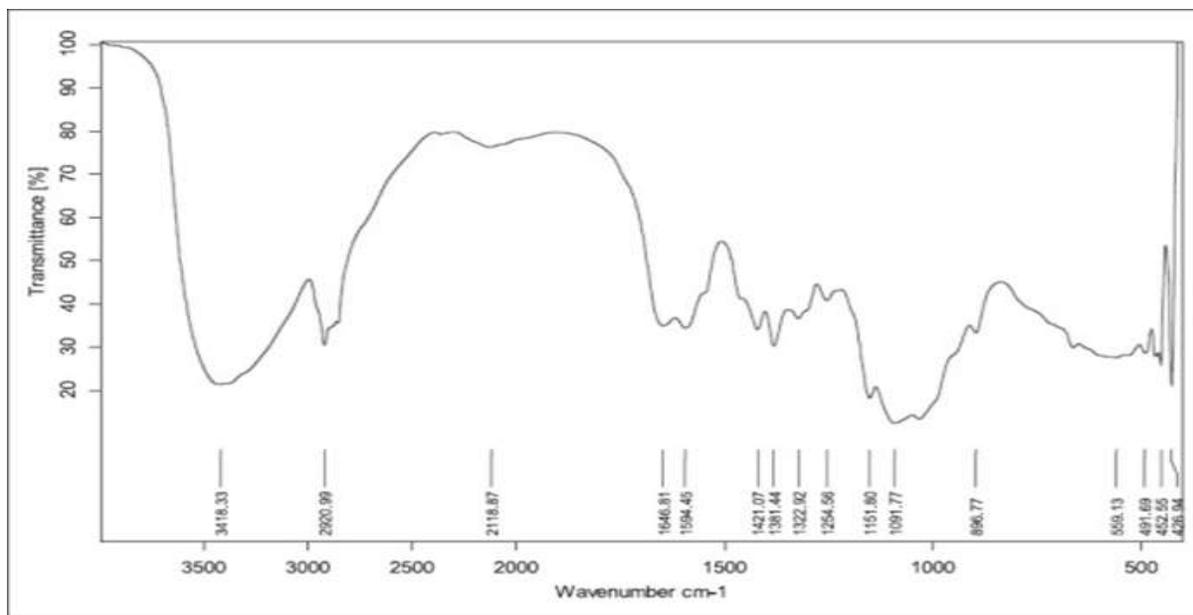
**Figure 3.** FTIR spectra of chitosan.
