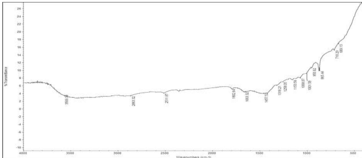
**Figure 2.** FTIR spectra of the chitin from shrimp shell.
