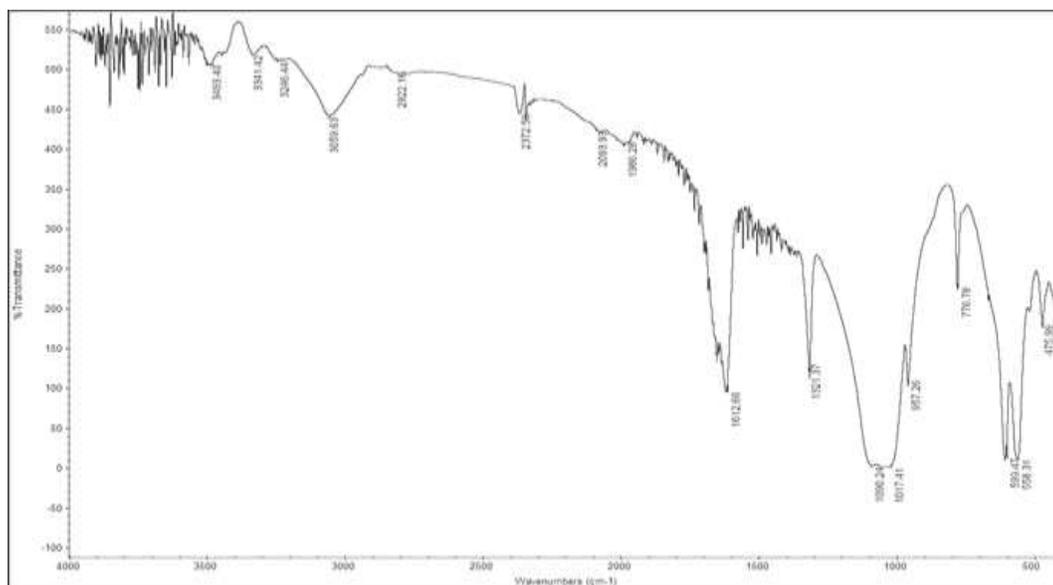
**Figure 11.** FTIR spectra of zinc (II) chloride-treated animal bone carbon impregnated on chitosan (ZABCC).**Table 9.** Characteristic absorption bands in the FTIR spectra of zinc (II) chloride-treated animal bone carbon impregnated on chitosan (ZABCC).
