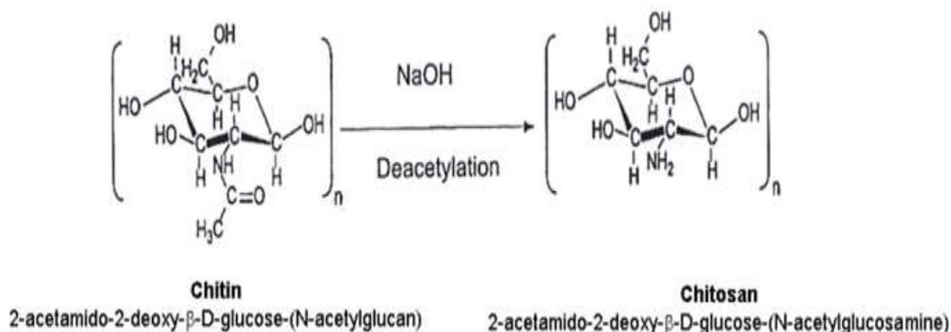
**Figure 1.** Chemical deacetylation of chitin to chitosan.
