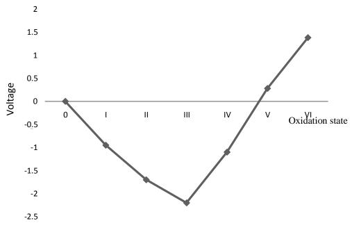
Figure 1. Oxidation state free energy diagram for chromium.
