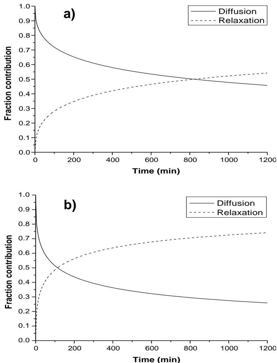
**Figure 7.** Fraction contribution of the Fickian diffusion and the erosion mechanisms (a) for formulation F2 ( $k_F = 0.01647 \text{ min}^{-0.447}$  and  $k_R = 0.00082 \text{ min}^{-0.894}$ ) and (b) for formulation F3 ( $k_F = 0.01262 \text{ min}^{-0.447}$  and  $k_R = 0.00152 \text{ min}^{-0.894}$ ).
