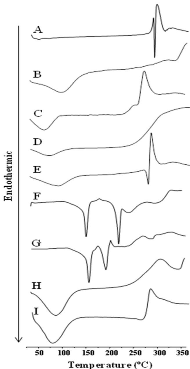
**Figure 1.** DSC curves of DS (A), HPMC K15M (B), DS:HPMC K15M (C), Chitosan (D), DS:Chitosan (E), LAC (F), DS:LAC (G), Chitosan:HPMC K15M (H), and DS:Chitosan:HPMC K15M (I) in 1:1 (C, E, G, and H) or 1:1:1 (I) (w/w) in the cases of physical mixtures.
