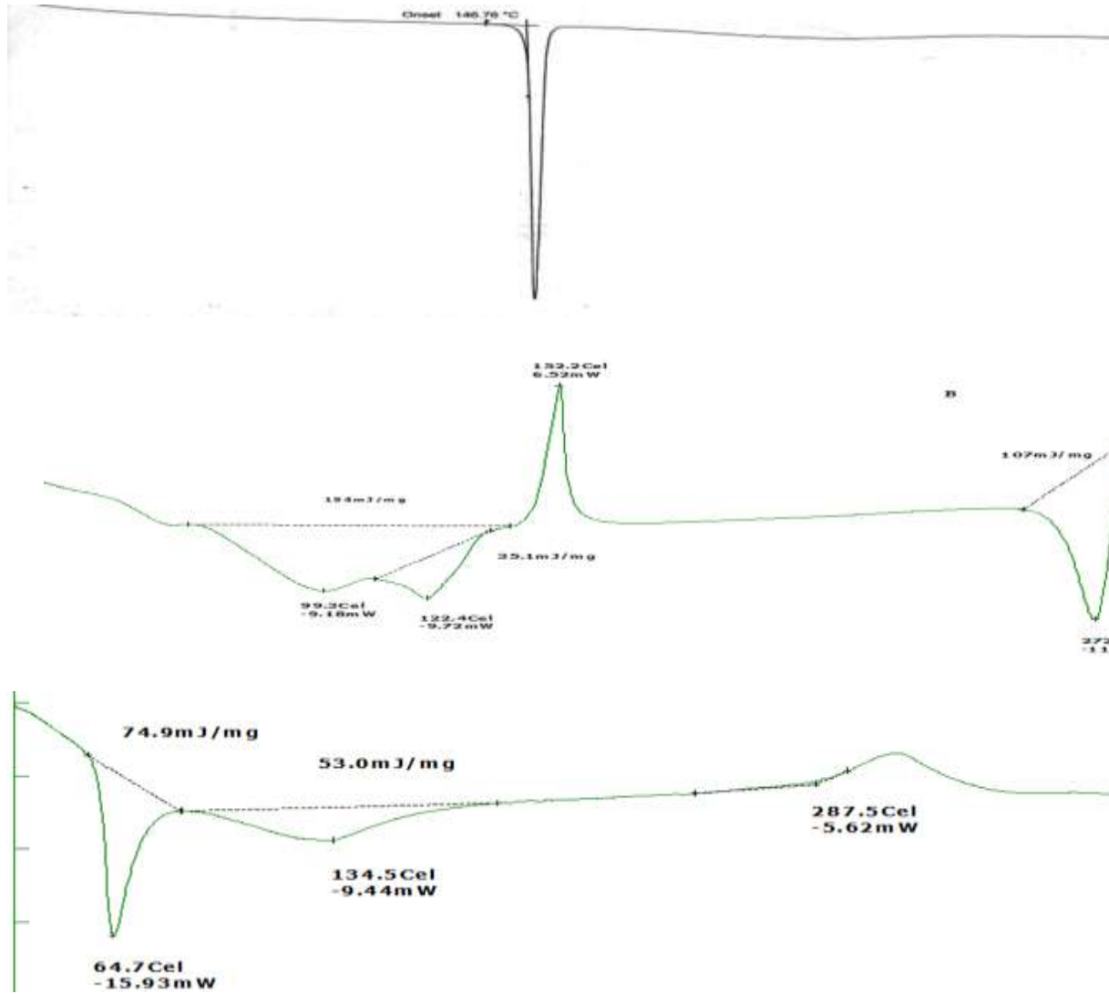
Figure 7. DSC of aceclofenac and its sodium alginate nanoparticles encapsulated gel.
