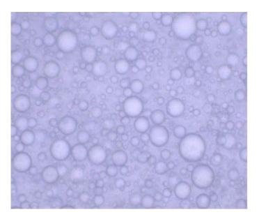
Figure 2. Photographs of microcapsules of Castor bean extract  $(\times 400)$ .
