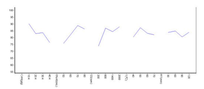
**Figure 1.** Effect of controllable factors on encapsulation efficiency. Y-axis: entrapment rate; X-axis: level of factor; C/W: core/wall (g/g); 5% A S: 5% acacia solution (ml); S S: stirring speed (rpm); T: temperature (); R T: reaction time (min).
