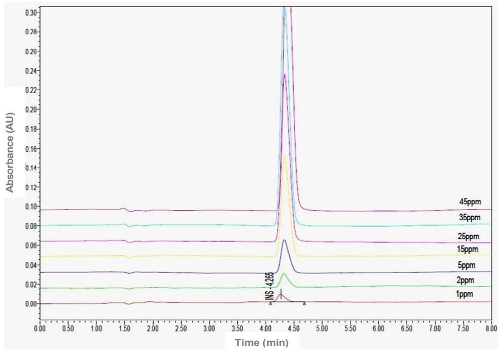
**Figure 1.** Chromatograms of Calibrators (10  $\mu$ l of standard solutions containing 1 to 45  $\mu$ g/ml of human insulin). Chromatograms of insulin Calibration standards on Symmetry<sup>®</sup> RP-C18 (150  $\times$  4.6 mm, 5 $\mu$ m). Regression equation;  $Y = 67755x + 10773$ , and correlation coefficient  $R^2 = 0.9997$
