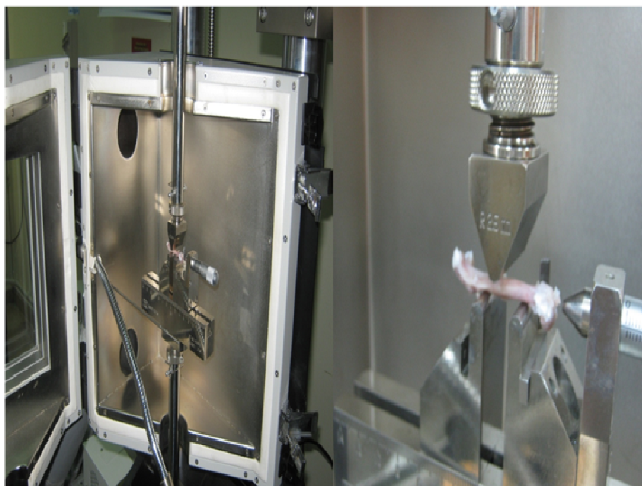
Figure 1. Photograph of three point bending test (Instron Microtester), showing preparation for biomechanical testing of fractured femur sample.
