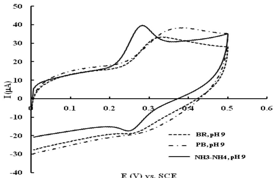
**Figure 2.** CVs obtained at GRPE with 0.5 mM paracetamol in different buffer solutions of pH 9.0.
