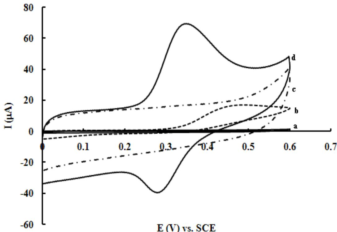
**Figure 1.** CVs at a bare CPE; (a) In the buffer of 0.1 M  $\text{NH}_3\text{-NH}_4\text{Cl}$ , pH 8.5; (b) a + 0.5 mM paracetamol; and at a GRPE (c) solution in (a); (d): solution in (b). Scan rate:  $50 \text{ mVs}^{-1}$ ; accumulation time: 120 s.
