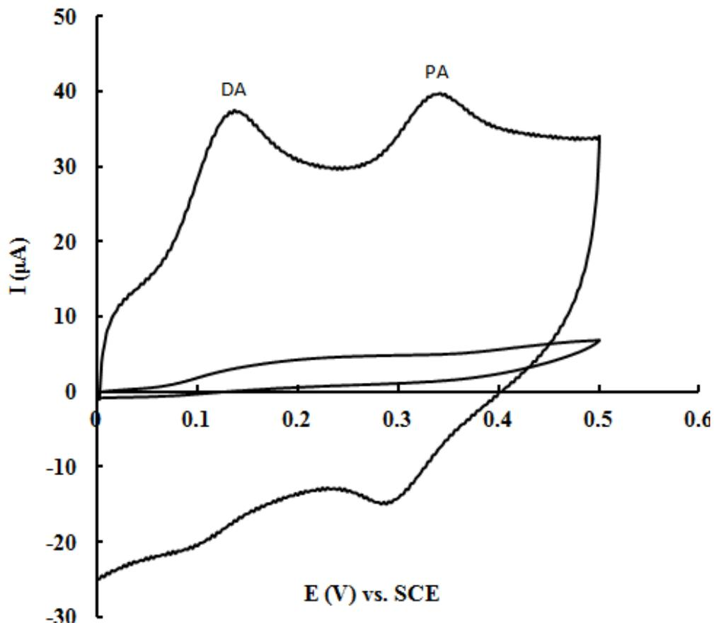
**Figure 6.** Cyclic voltammograms for a mixture of paracetamol (0.1 mM) and dopamine (0.1 mM) on a bare carbon paste electrode (lower) and a GRPE (upper).
