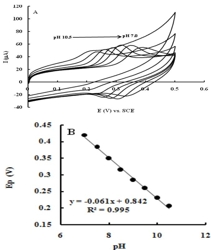
**Figure 3.** A: CVs obtained at GRPE with 0.2 mM paracetamol in 0.1 M  $\text{NH}_3\text{-NH}_4\text{Cl}$  buffers with pH values of 7.5, 8.0, 8.5, 9.0, 9.5, 10.0 and 10.5; B: Plot of oxidation peak potentials versus pH values of the solution. Scan rate:  $50 \text{ mVs}^{-1}$ .
