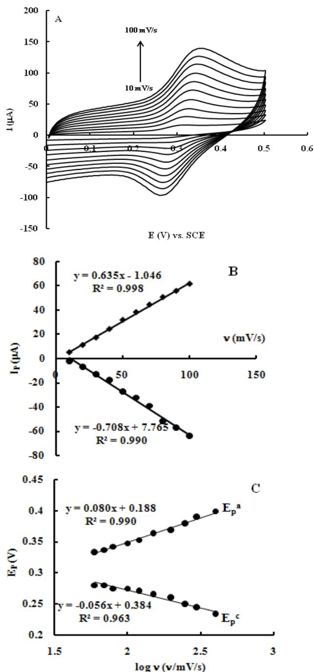
**Figure 4.** CVs acquired on GPE with 0.2 mM paracetamol in the buffer of  $\text{NH}_3\text{-H}_2\text{O-NH}_4\text{Cl}$  (0.1 M pH 8.5) at different scan rates from 10 to 100  $\text{mVs}^{-1}$ . Inset is the plot of the peak current of paracetamol versus scan rate.
