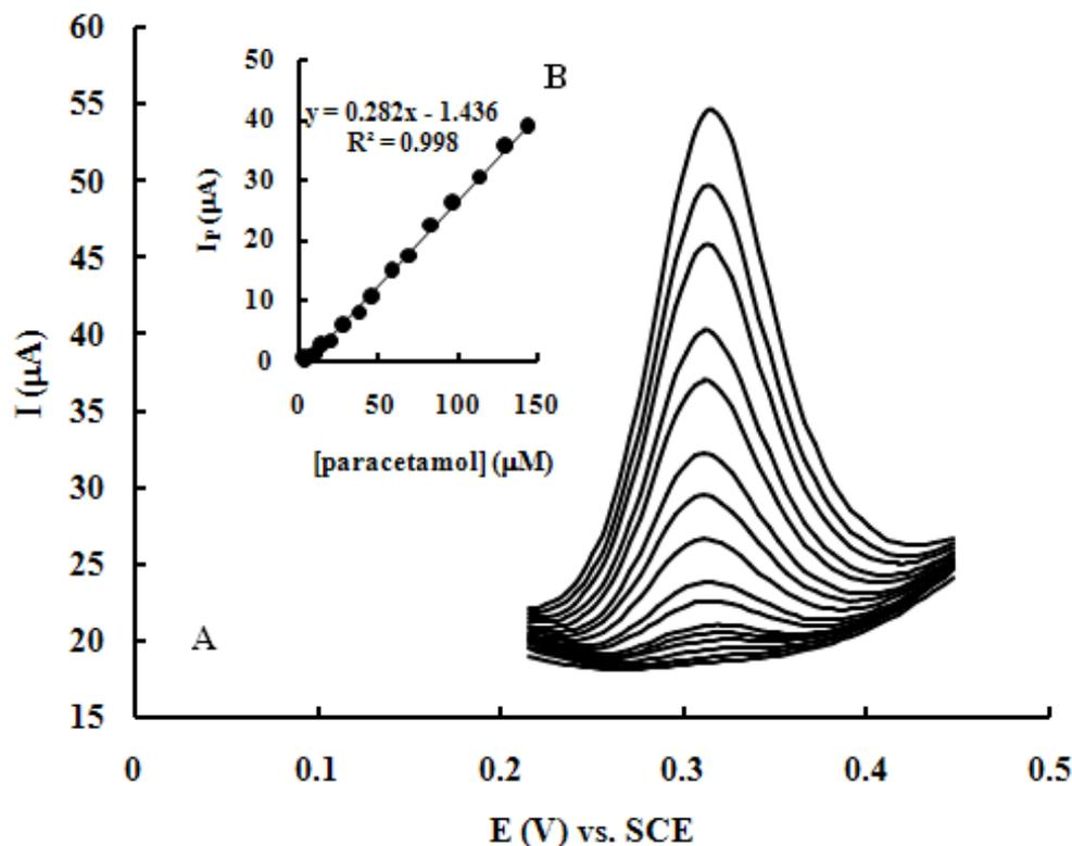
**Figure 5.** A: SWVs on GRPE for different paracetamol concentrations; from bottom: 0.0, 2.5, 3.5, 5.0, 7.4, 9.8, 14.6, 19.2, 28.3, 37, 45.5, 57.5, 69, 83.3, 96.8, 112, 130, and 143  $\mu\text{M}$  in 0.1 M  $\text{NH}_3\text{-NH}_4\text{Cl}$ . B: Calibration plot.
