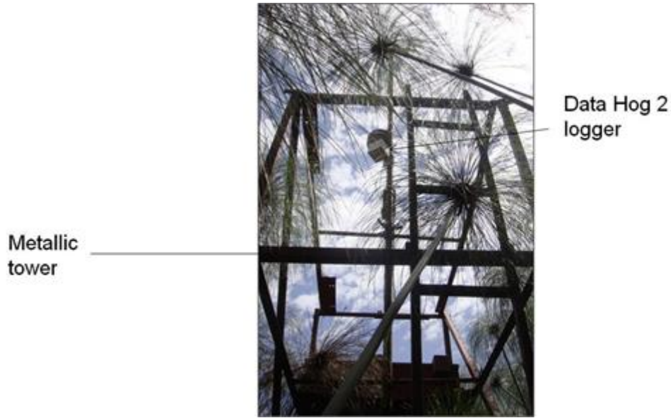
Figure 1. Mounted metallic tower in Lubigi wetland. On top are Data Hog 2 logger, anemometer and pyranometer. The pyranometer and anemometer are obscured by papyrus umbel structures.
