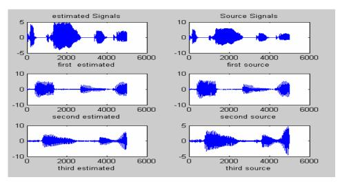
Figure 3. The estimated signals in left with scales, permutation and original signals in right.
