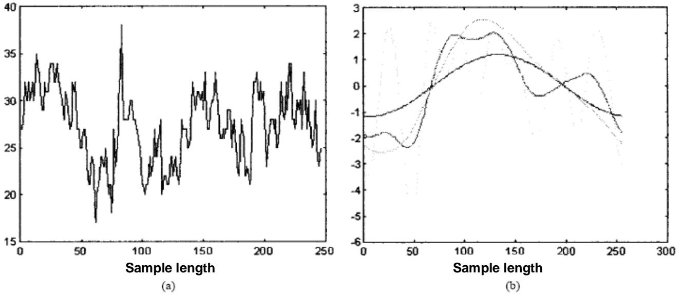
Figure 3. (a) Sample iris signature from the image of Figure 1. (b) Lowest four resolution levels of the wavelet transform.
