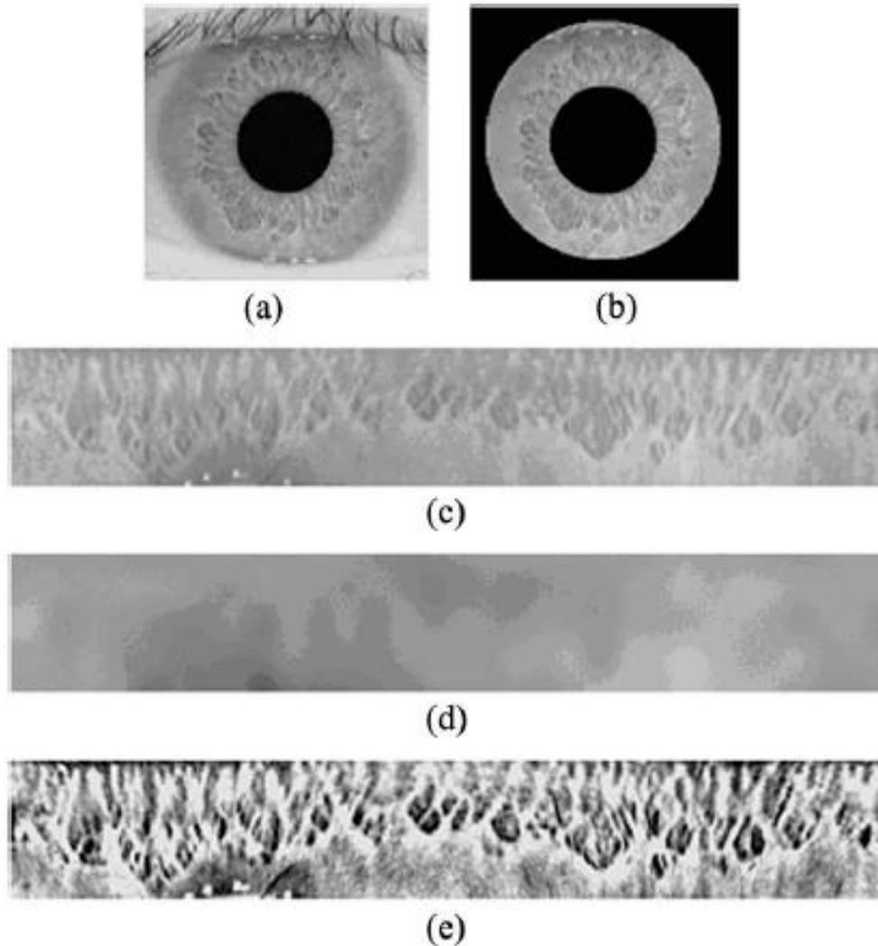
**Figure 5.** Iris image preprocessing: (a) original image; (b) localized image; (c) normalized image; (d) estimated local average intensity; and (e) enhanced image.
