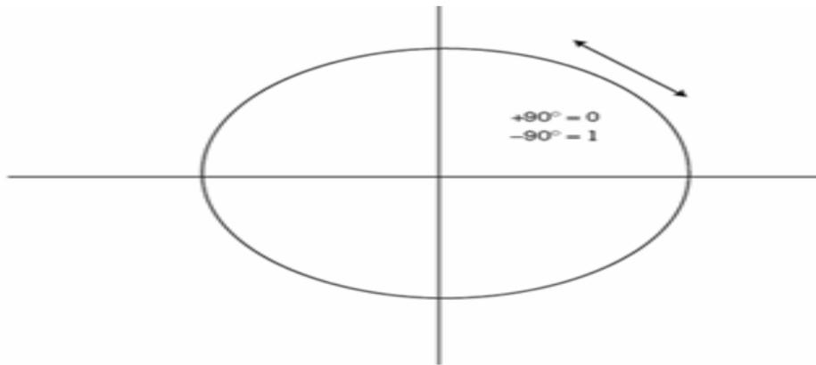
**Figure 4.** GSM uses GMSK modulation. Amplitude remains constant during phase shifts of  $\pm 90^\circ$ . The constellation of a GSM signal thus resembles a circle. Andrew (2003).
