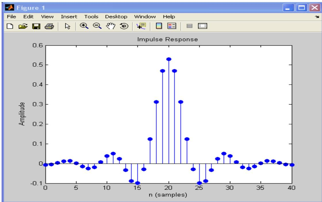
Figure 9. Square root raised cosine filter used in QPSK modulation technique.
