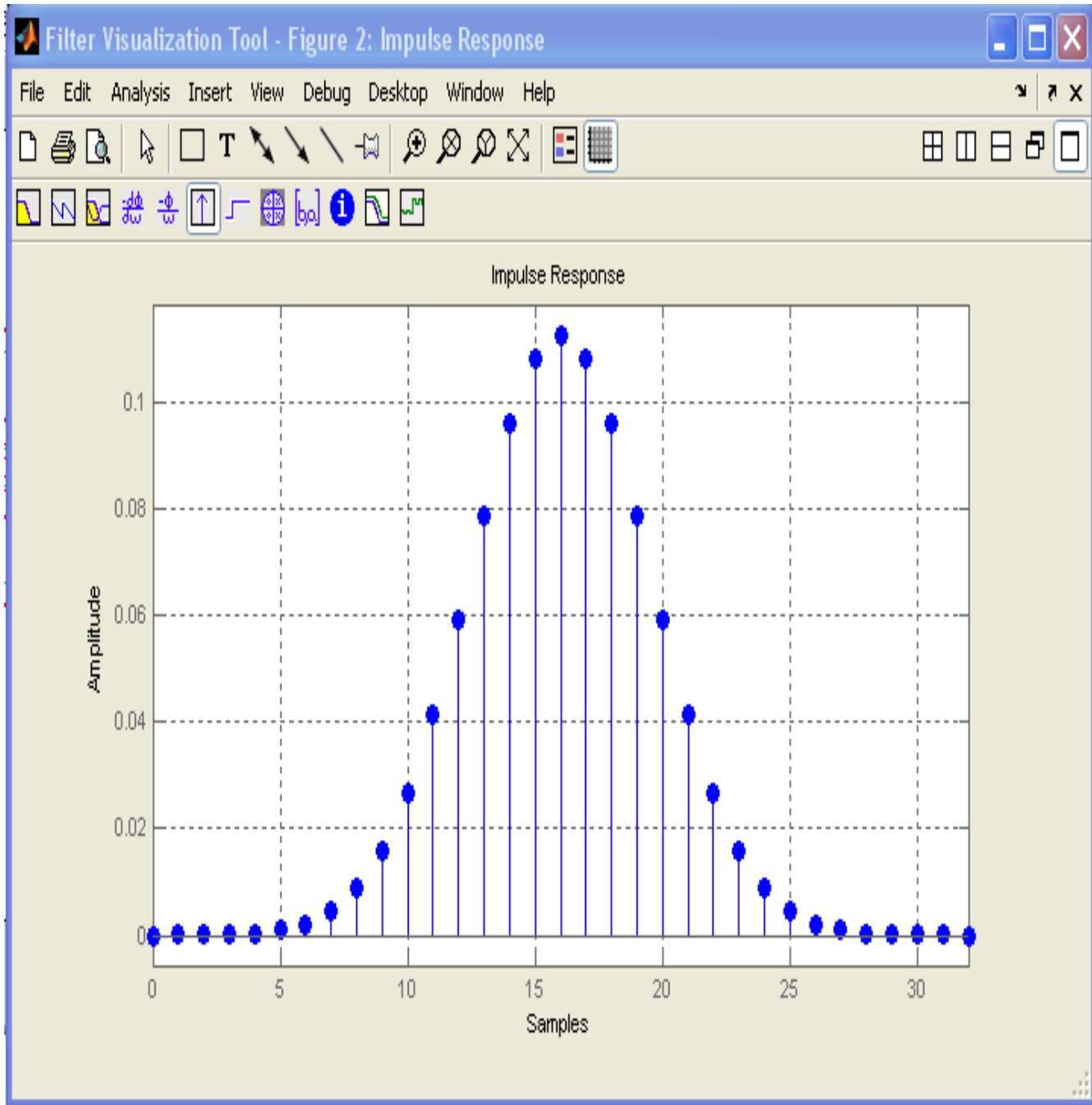
Figure 7. Gaussian pulse-shaping Filter used in GMSK modulation technique.
