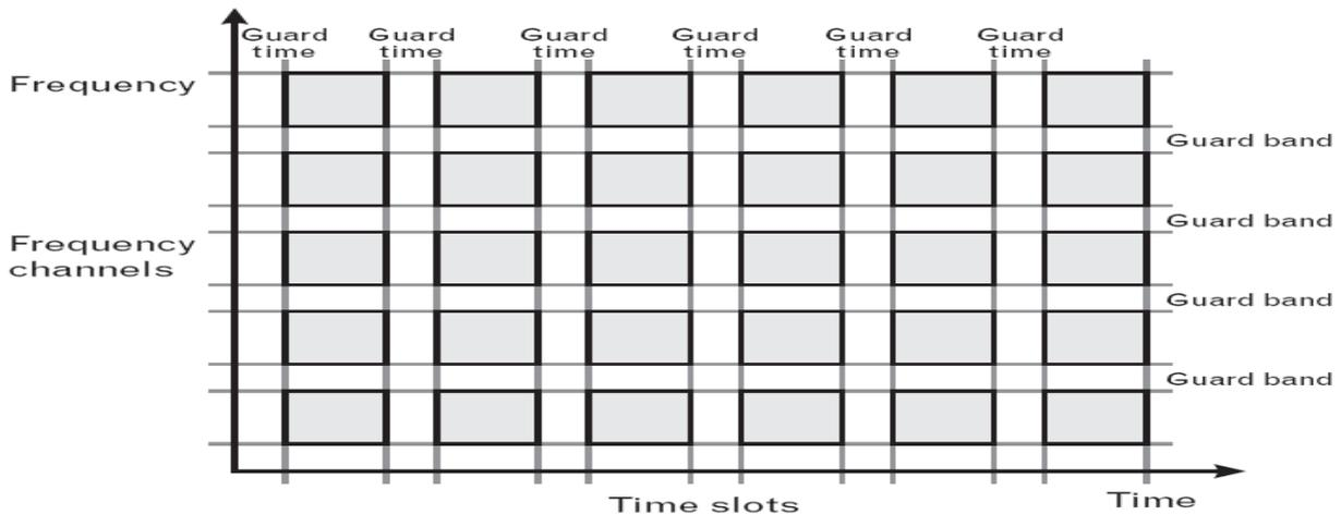
**Figure 1.** Hybrid frequency division multiple access/ time division multiple access (FDMA/TDMA) system. Korhonen (2003).
