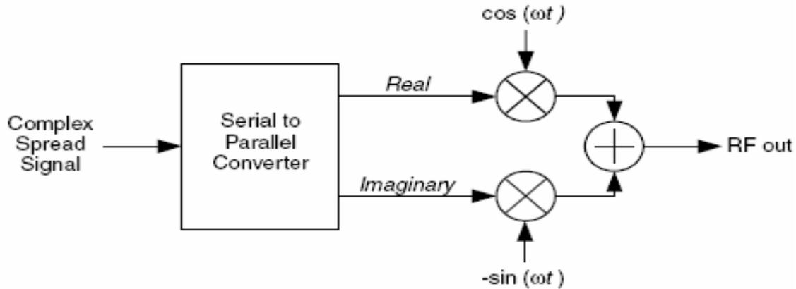
**Figure 3.** QPSK modulation principle. This modulation technique is used in 3G system. Jeffrey et al. (2004)
