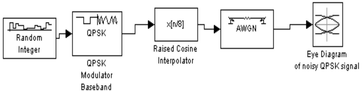
**Figure 5.** Block diagram of QPSK transmitter. The quadrature form of modulating using I and Q channel.
