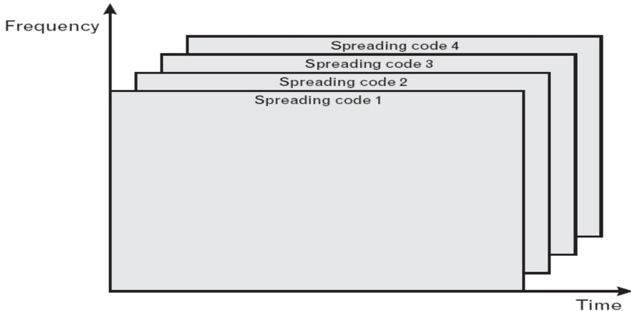
**Figure 2.** CDMA system: all users occupy the same frequency at the same time, but their signals are separated from each other by means of special codes. Korhonen (2003).
