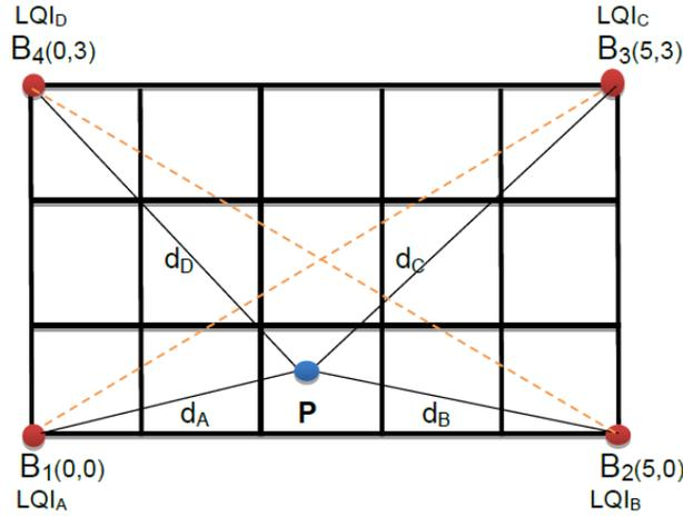
**Figure 4.** 5 × 3 m test area with  $B_i$  transmitters and  $P$  unknown mobile node.
