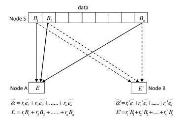
Figure 4. Data encoding at the relay node.
