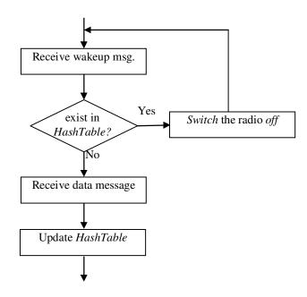
Figure 9. The flowchart of packet reception with overhearing avoidance.
