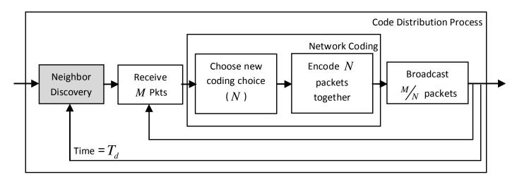
Figure 2. The code distribution process in AdapCode+.
