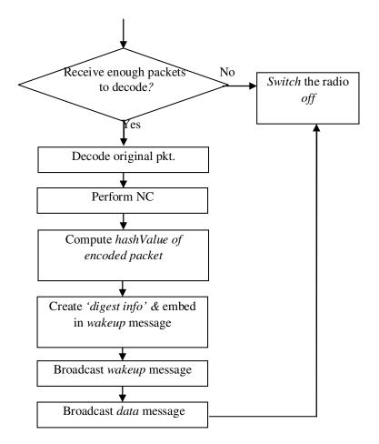
Figure 10a. The flowchart of packet transmission.
