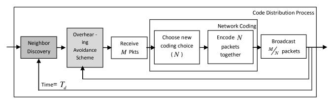
Figure 7. The code distribution process in AdapCode++.
