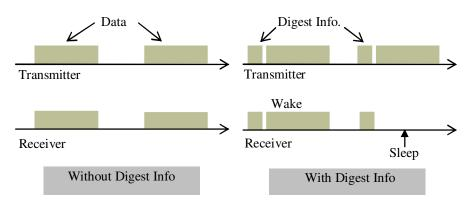
Figure 8. Avoiding overhearing of redundant message by means of 'Digest Info'.
