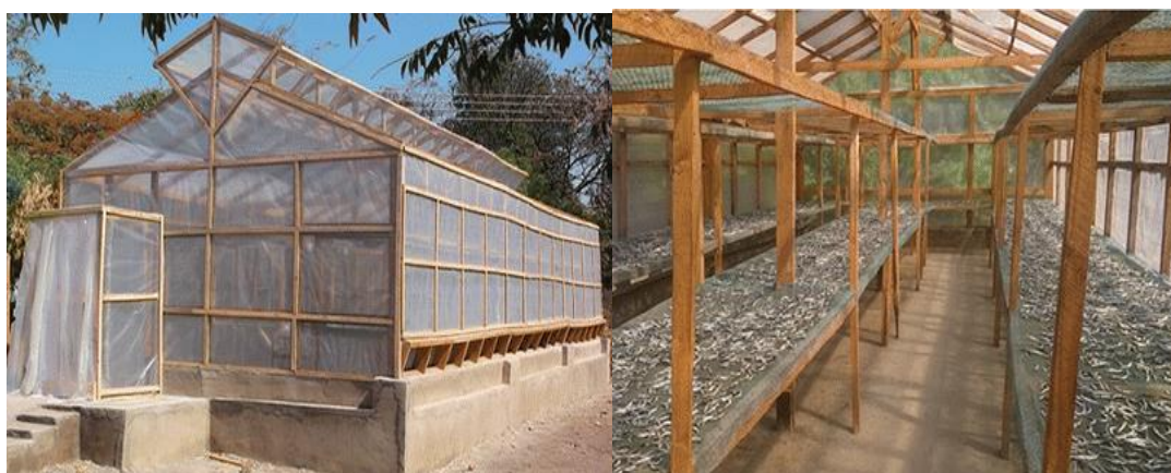
Figure 3. Solar tent dryer (left) used by the study and the inside view. Besides problems with air vents to allow easy circulation of air, no black surface was placed inside to help with heat absorption in this design.
