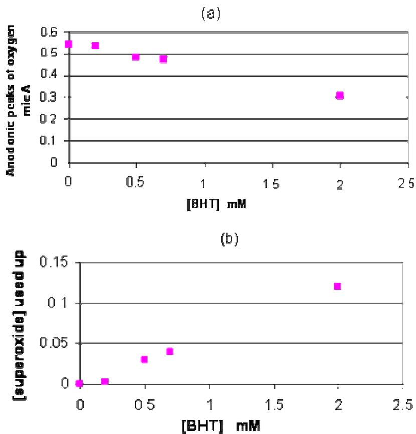
Figure 7. Calibration curves: (a) BHT concentration vs. anodic peaks of  $\text{O}_2$ ; (b) BHT concentration vs.  $\text{O}_2^{\cdot-}$  used up. Concentrations in mM.
