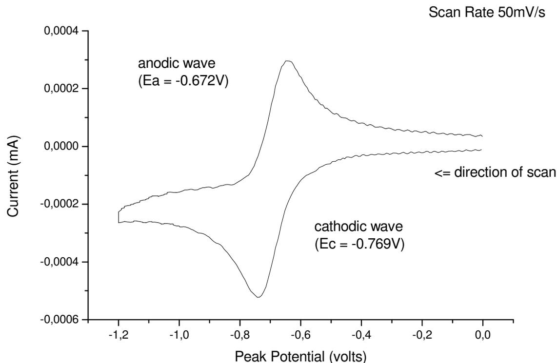
**Figure 1.** Cyclic voltammogram of  $O_2/O_2^-$  in DMSO (0.1 TBAI); working electrode = Glassy carbon, reference electrode = gold wire QRE, counter electrode = platinum wire.
