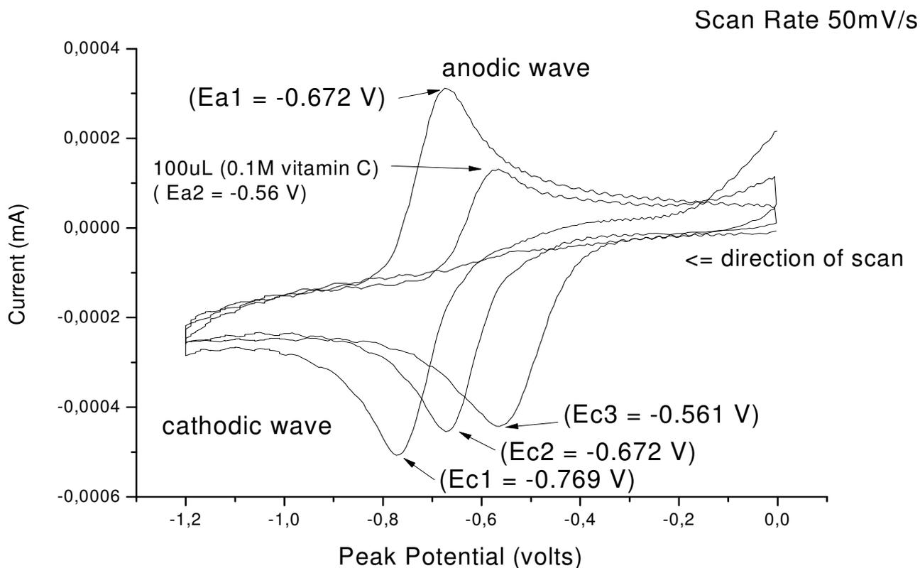
Figure 4. Cyclic voltammogram of  $O_2/O_2^-$  in the presence of vitamin C; condition same as in Figure 1.
