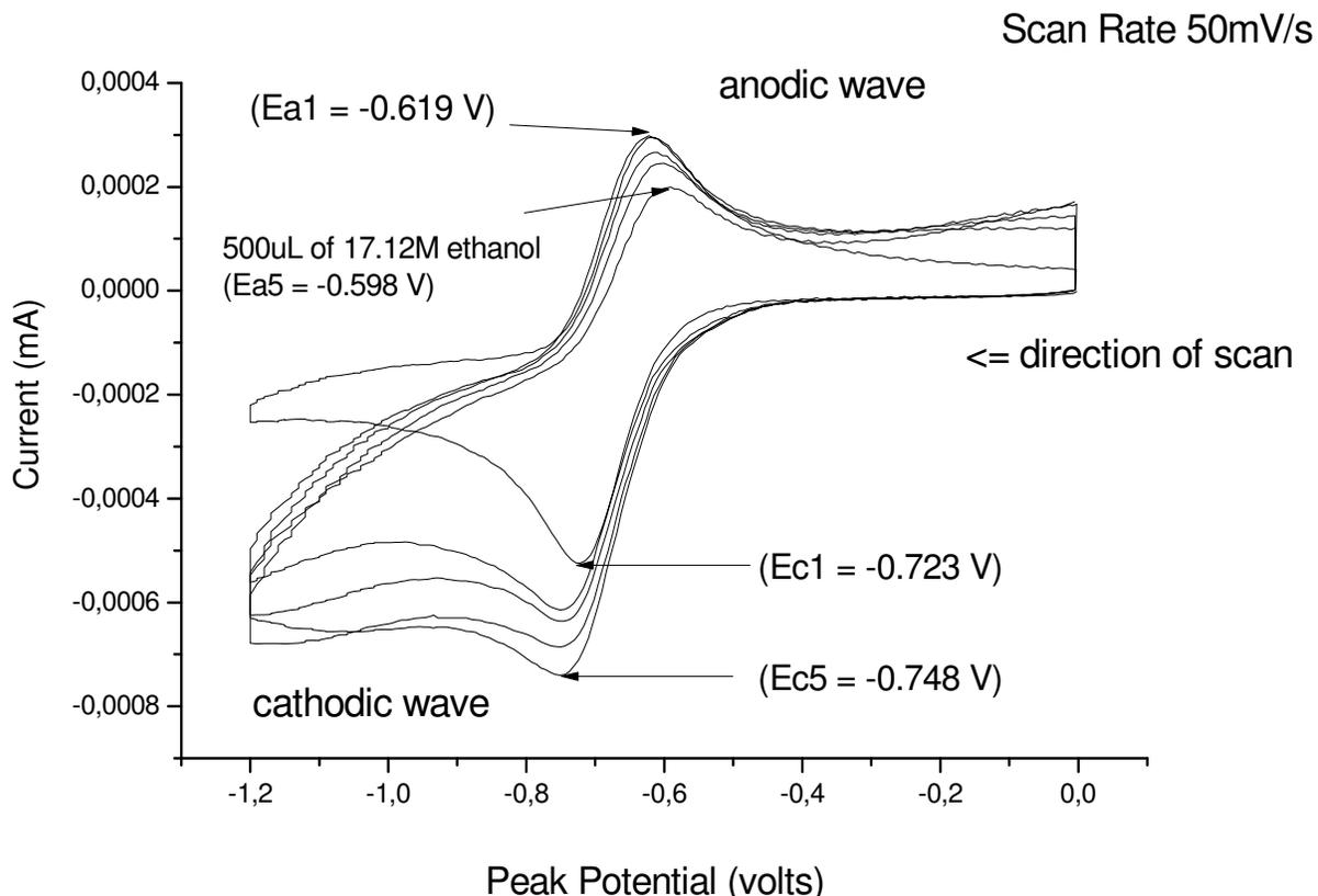
**Figure 3.** Cyclic voltammogram of  $O_2/O_2^-$  in the presence of ethanol; condition same as in Figure 1.
