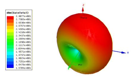
Figure 4. Radiation pattern of PSA.
