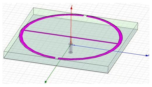
Figure 1. Structure of the phi shaped antenna.
