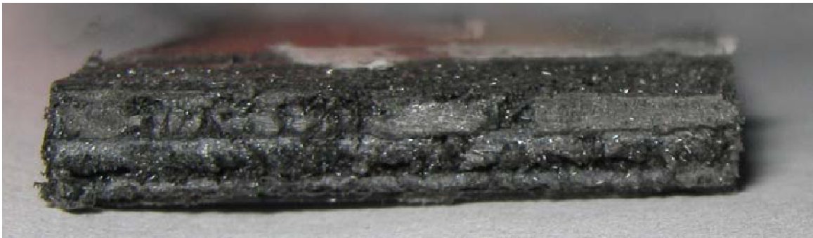
Figure 7. Tunnel defect in stir zone.
