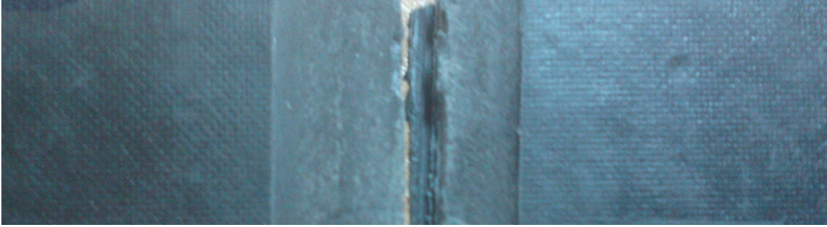
Figure 6. The tensile test fractured specimen.
