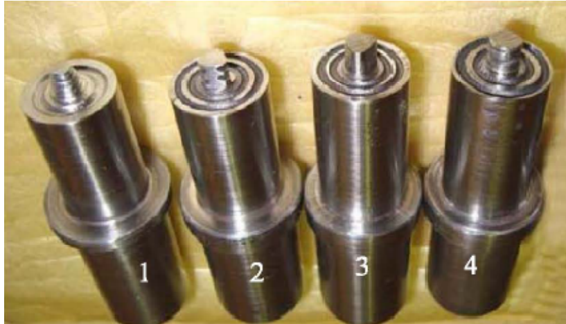
Figure 2. FSW tools with different pins and shoulders.
