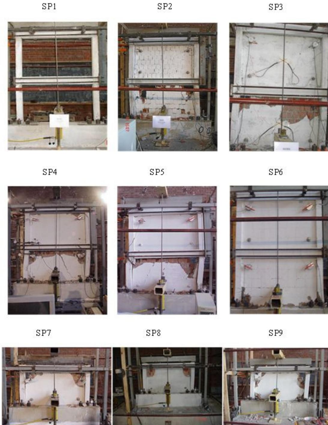
Figure 7. Test frames after failure.
