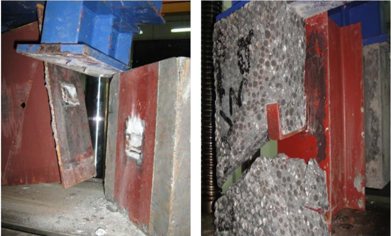
Figure 2. Typical types of failure for channel connectors (left: concrete crushing-splitting, right: channel fracture).
