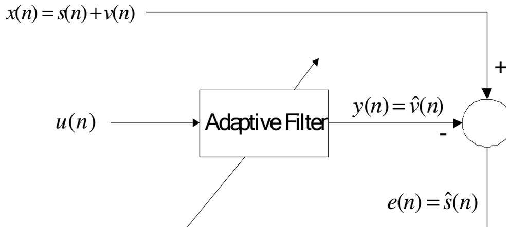
Figure 1. General model of ANC with reference input.
