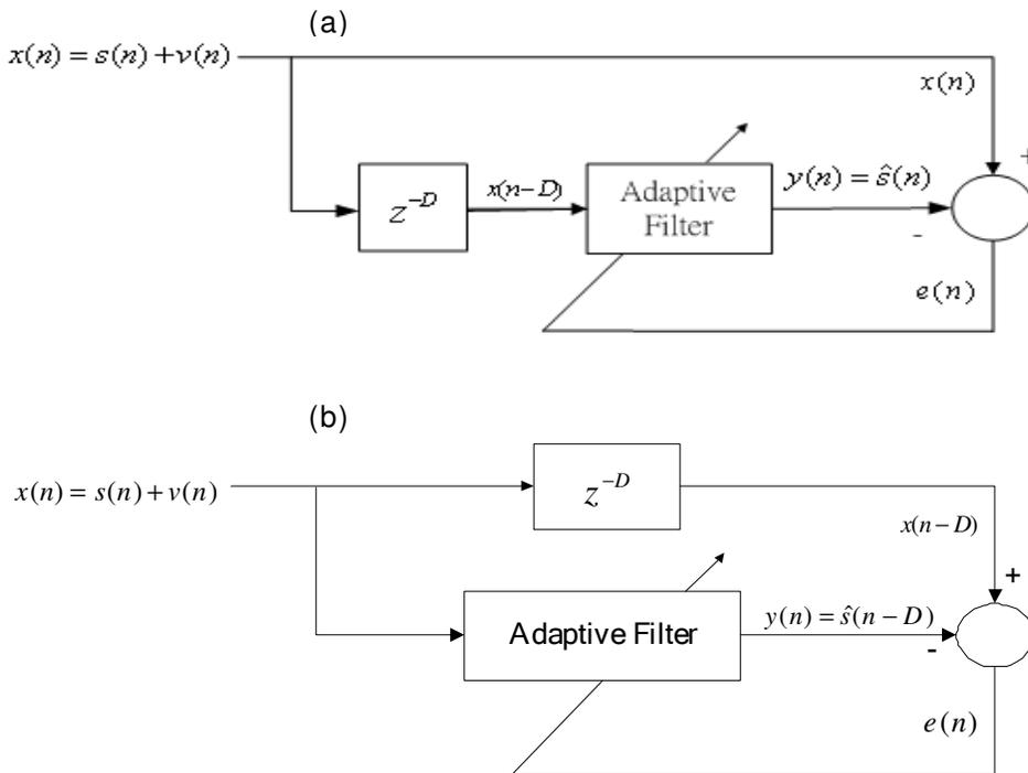
Figure 3. SIANC with delays inserted in the paths of (a) reference input and (b) primary input.
