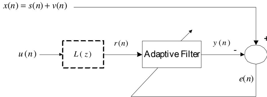
Figure 2. ANC with limited availability on the reference input.
