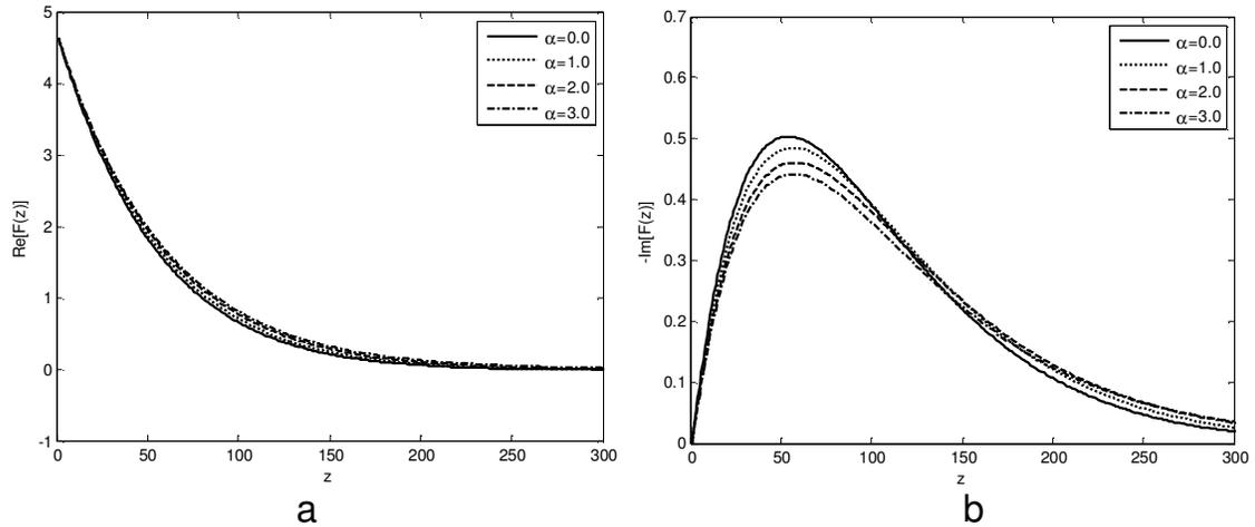
**Figure 3.** Profiles of the normalized steady state velocity  $F(z)$  for various values of  $\alpha$  when  $(A=.5, M = 2, P = 1, \Omega = 1, t = 2\pi)$ .
