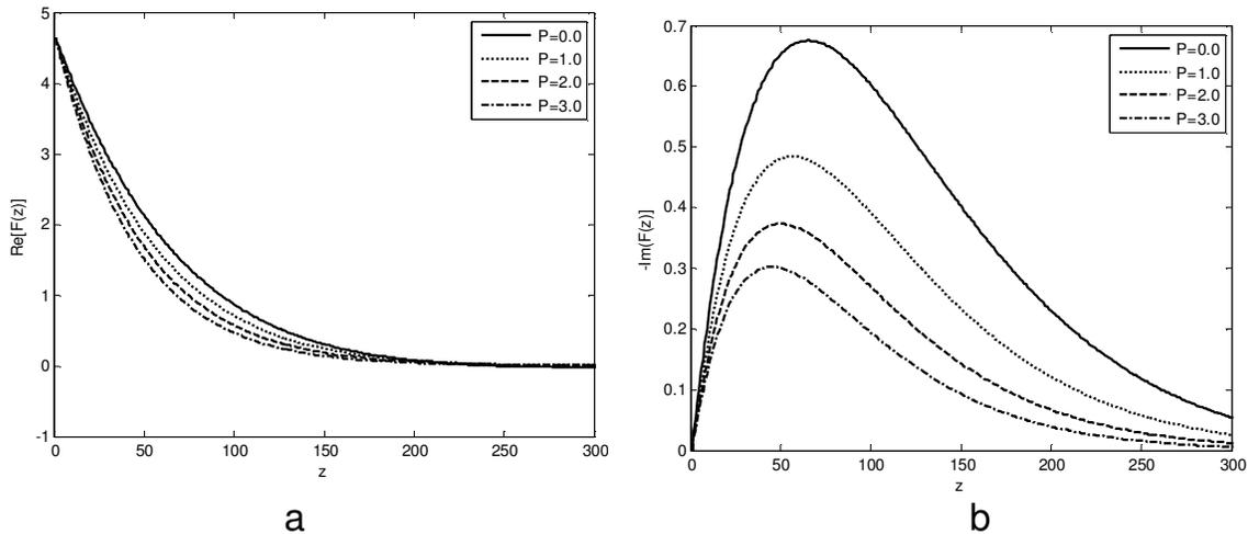
**Figure 4.** Profiles of the normalized steady state velocity  $F(z)$  for various values of  $P$  when  $(A=.5, \alpha = 1, M = 2, \Omega = 1, t = 2\pi)$ .
