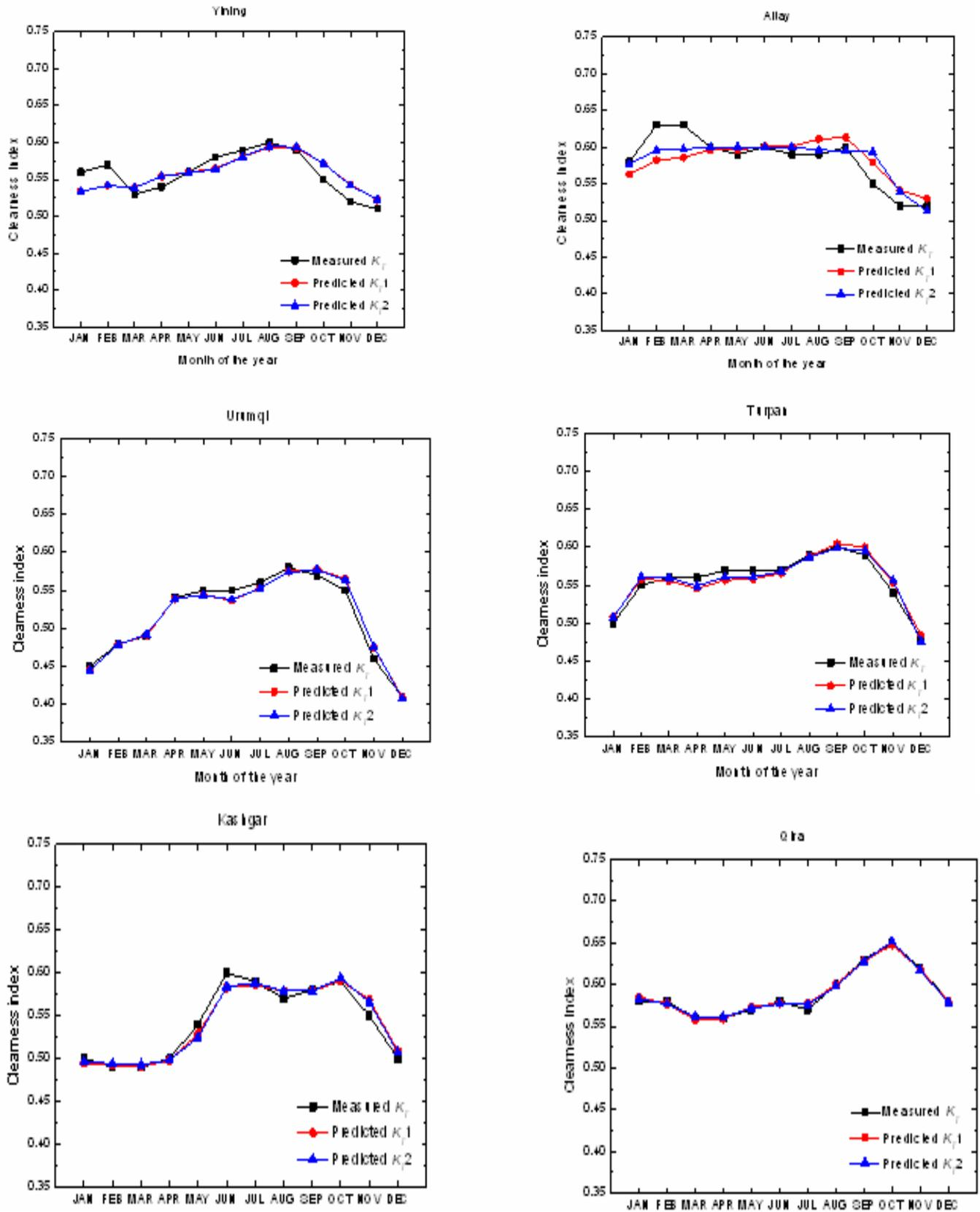
Figure 3. The measured monthly mean  $K_T$  and the simulated ones by using linear (Predicted  $K_{T1}$ ) and quadratic (Predicted  $K_{T2}$ ) fitting functions.
