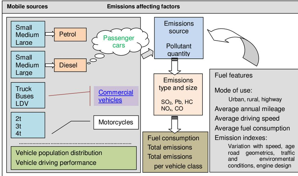
Figure 1. Procedure for estimating motor vehicle emission index.
