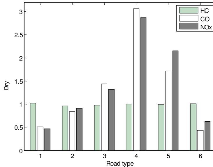
**Figure 4.**  $\lambda_{rp}$  determination as grade ratio of traffic air pollution. Notation for road type: 1: expressway; 2: major arterial; 3: minor arterial; 4: branch and minor street; 5: suburb highway; 6: suburb freeway.
