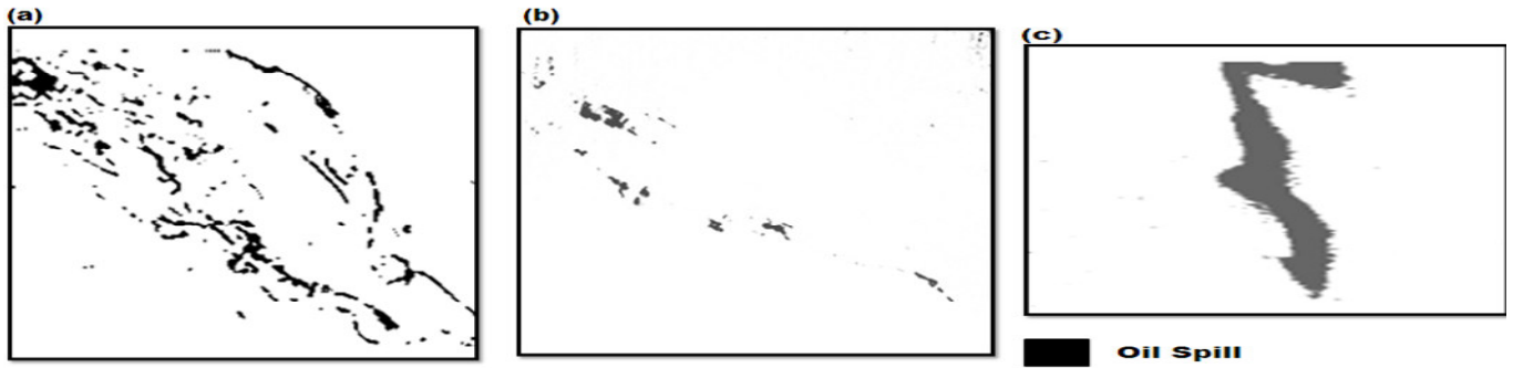
Figure 4. Oil spill detection using entropy algorithm with kernel window size 7 \times 7 pixels and lines in W1, S1 and S2 mode data.
