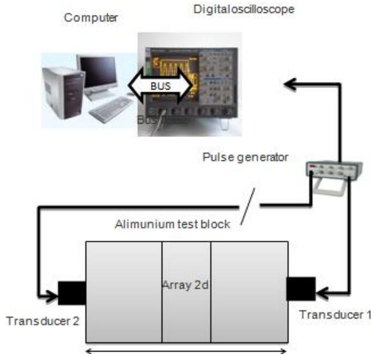
Figure 5. Experimental device.
