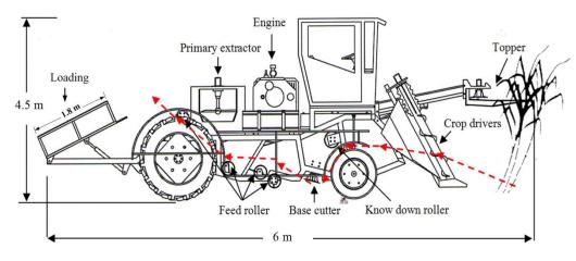
Figure 1. The component of the sugarcane harvester.
