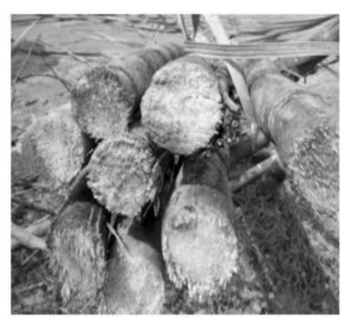
Figure 5. A smooth trace of each cut stump from cutting blade.
