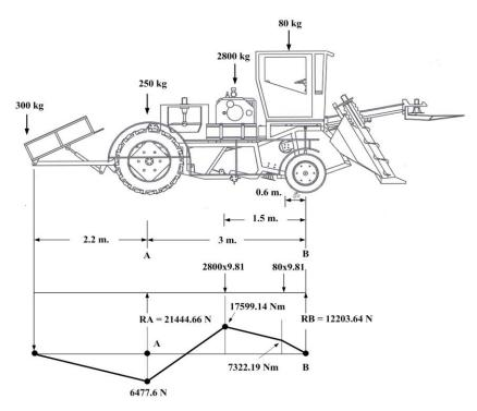
Figure 2. Shear and moment diagrams of beams.
