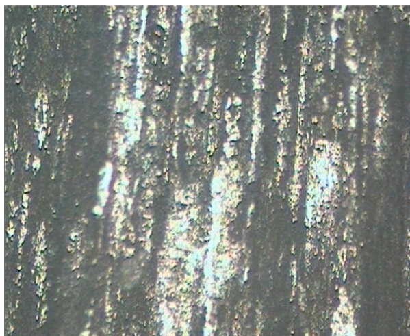
Figure 4a. -Mild steel sample blank kept in 1 M HCl for 24 h at 35°C.
