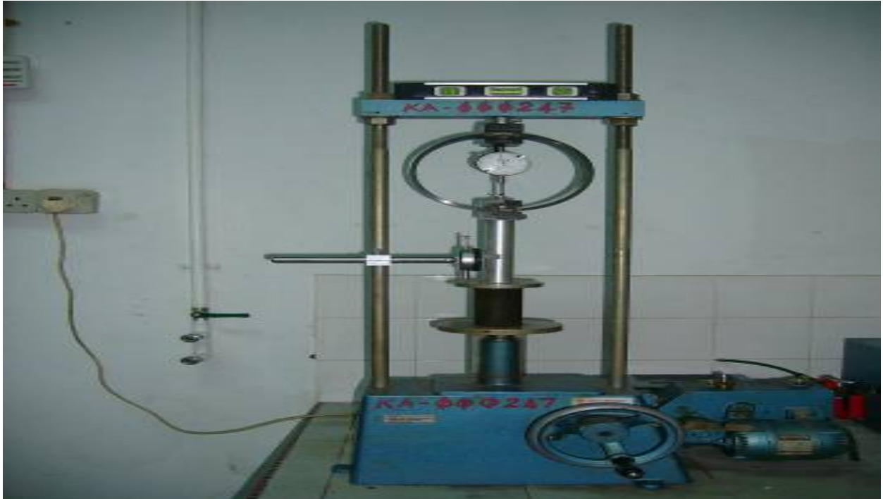
Figure 1. Unconfined compression test using 4.5 kN ELE proving ring.
