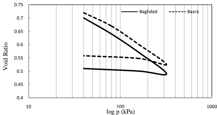
**Figure 3.** Void ratio versus log p (applied pressure) for untreated soils.
