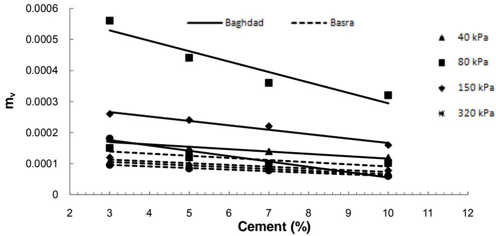
Figure 17. Coefficient of volume change versus cement content for 14 days curing period.
