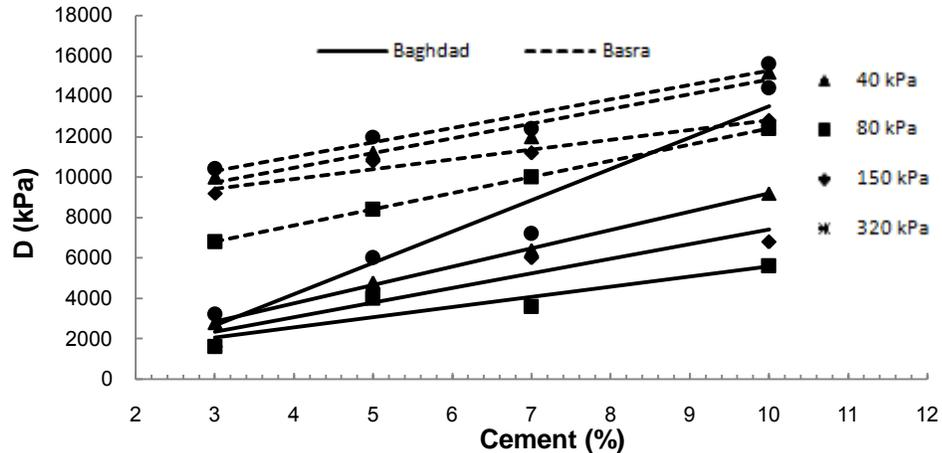
Figure 20. Concentrated modulus versus cement content for 14 days curing period.
