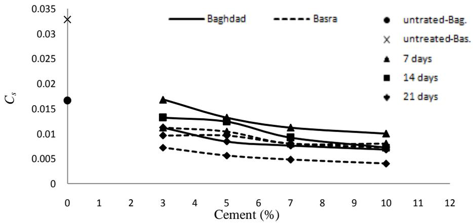
Figure 8. Swelling index versus cement content.
