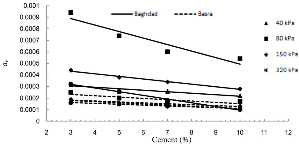
Figure 14. Coefficient of compressibility versus cement content for 14 days curing period.
