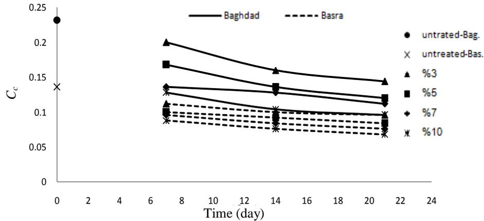
Figure 10. Compression index versus time.
