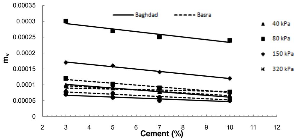
Figure 18. Coefficient of volume change versus cement content for 21 days curing period.
