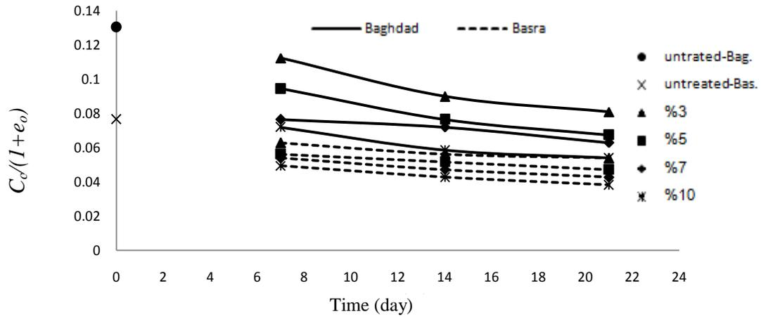
Figure 12. Compression ratio versus time.
