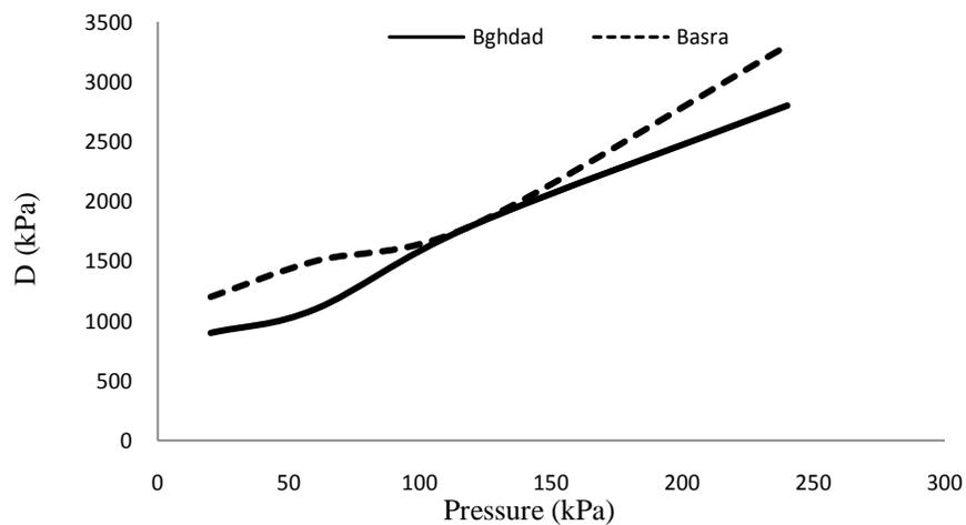
**Figure 6.** Constrained modulus versus applied pressure.
