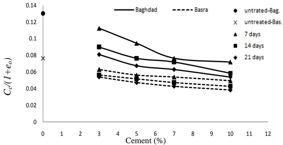
Figure 9. Compression ratio versus cement content.
