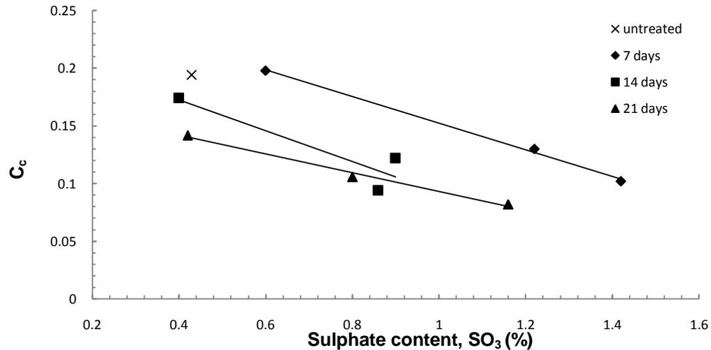
Figure 26. Compression index versus sulphate content.
