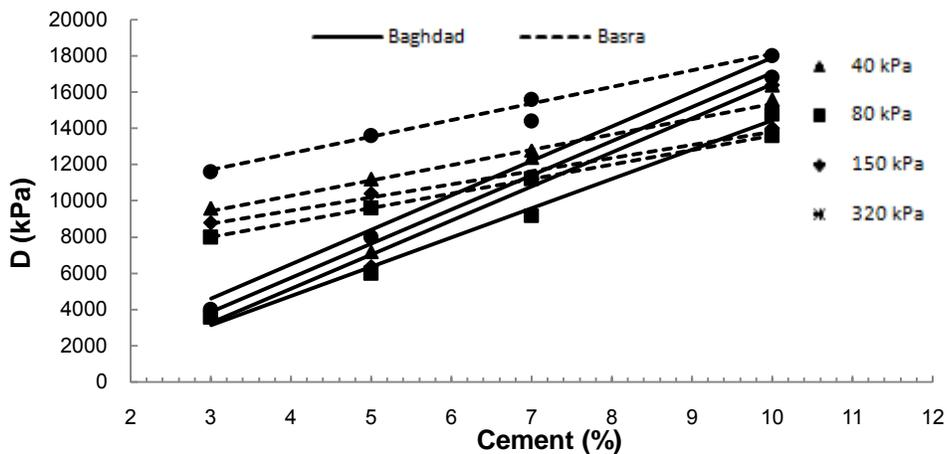
Figure 21. Concentrated modulus versus cement content for 21 days curing period.
