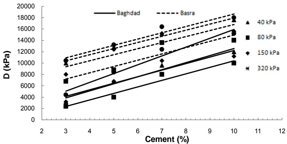
Figure 19. Concentrated modulus versus cement content for 7 days curing period.
