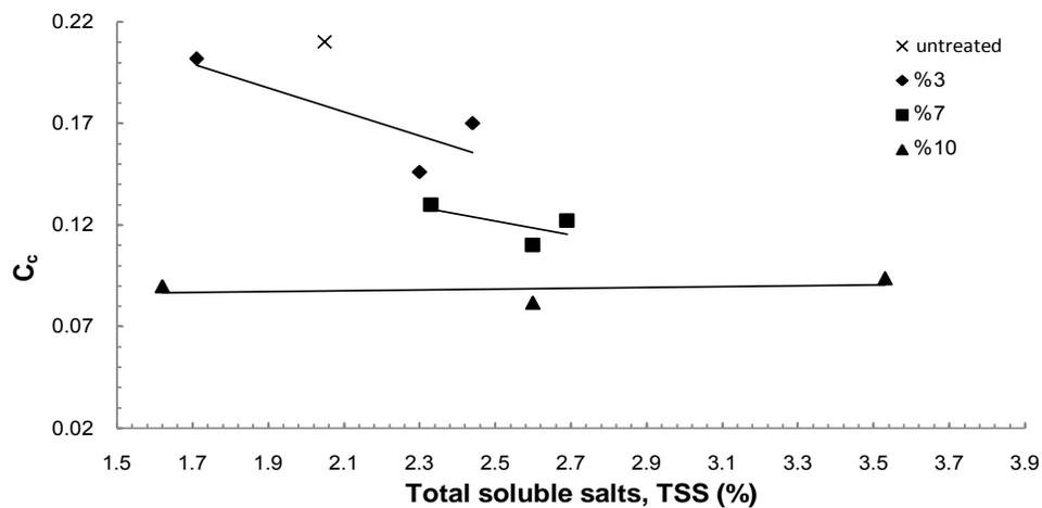
**Figure 24.** Compression index versus total soluble salts.
