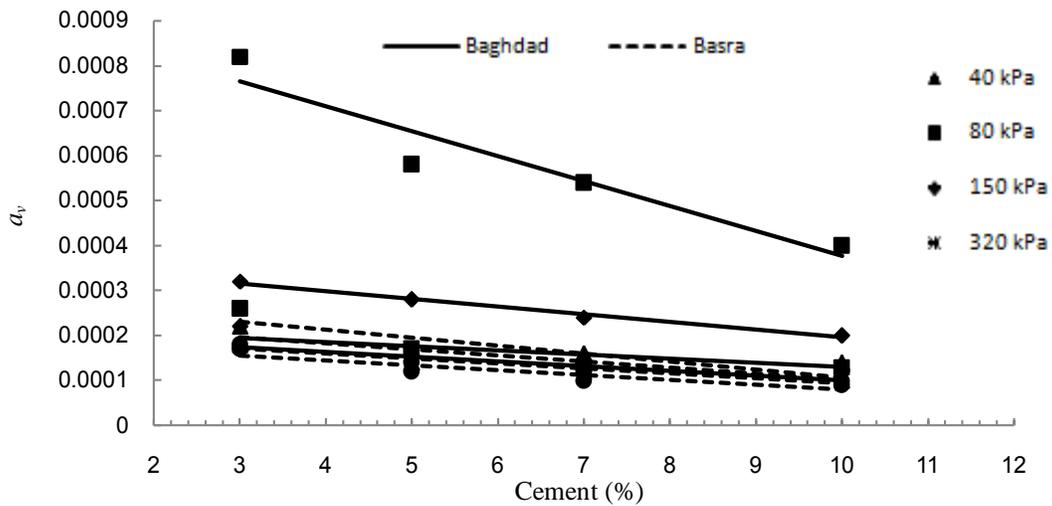
Figure 13. Coefficient of compressibility versus cement content for 7 days curing period.
