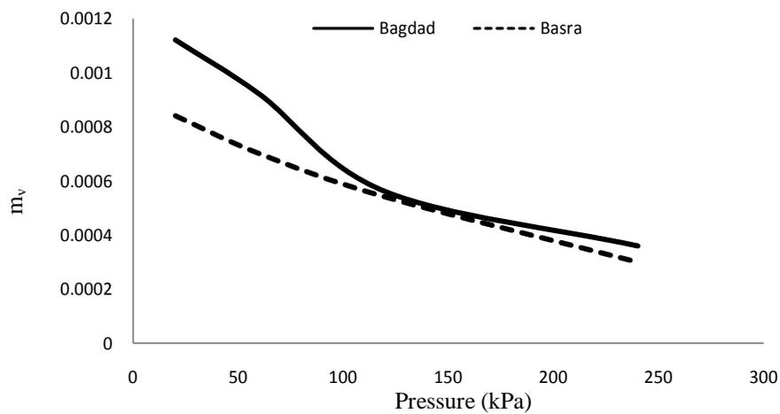
**Figure 5.** Coefficient of volume change versus applied pressure.
