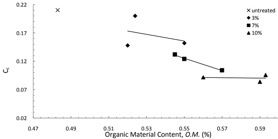
**Figure 23.** Compression index versus organic material content.
