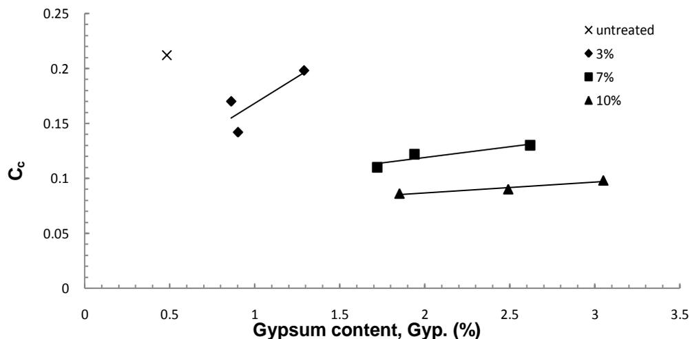
**Figure 22.** Compression index versus gypsum content.
