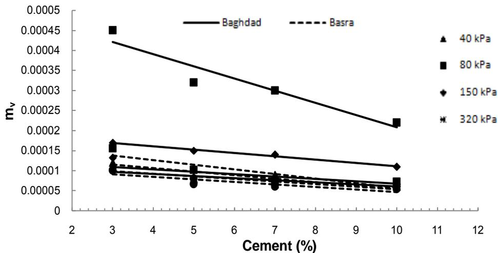
**Figure 16.** Coefficient of volume change versus cement content for 7 days curing period.
