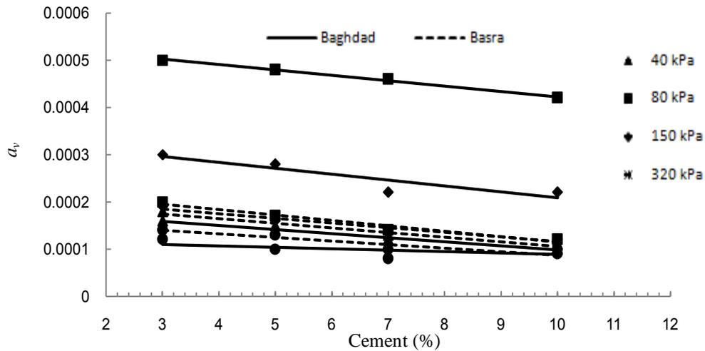
**Figure 15.** Coefficient of compressibility versus cement content for 21 days curing period.
