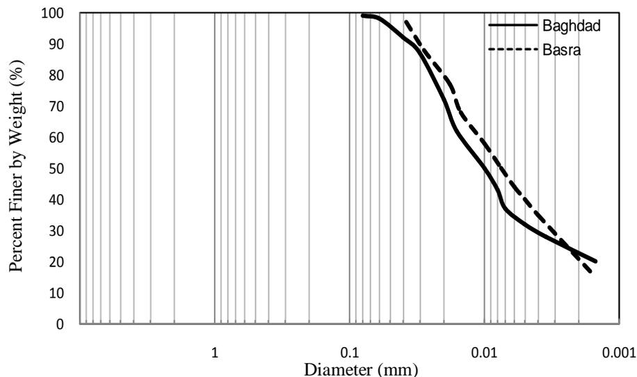
Figure 2. Grain size distribution of soils.
