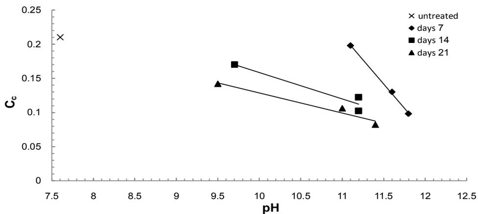
**Figure 25.** Compression index versus pH value.
