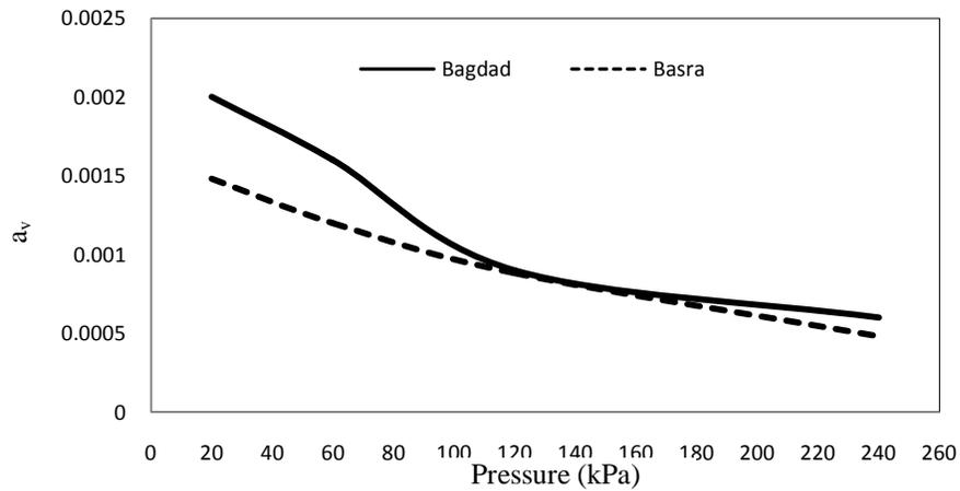
**Figure 4.** Coefficient of compressibility versus applied pressure.
