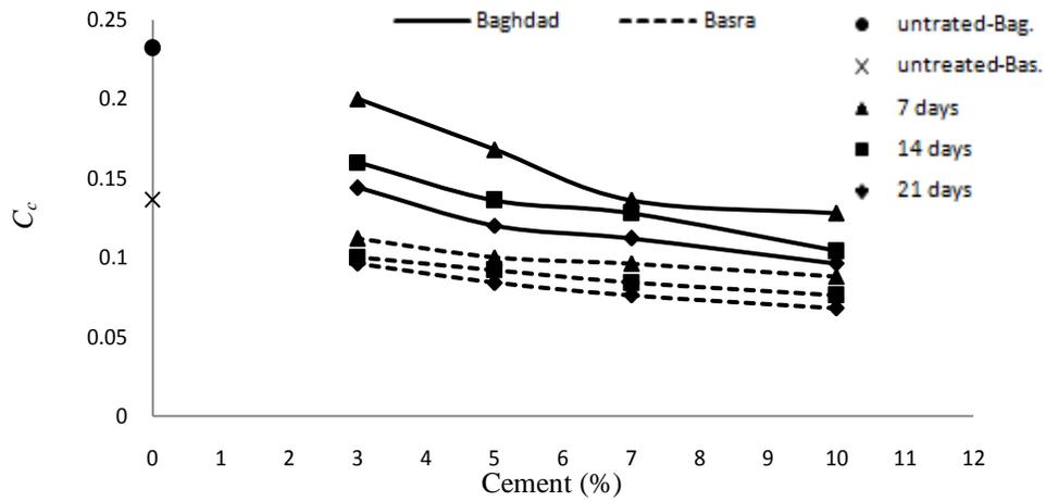
Figure 7. Compression index versus cement content.
