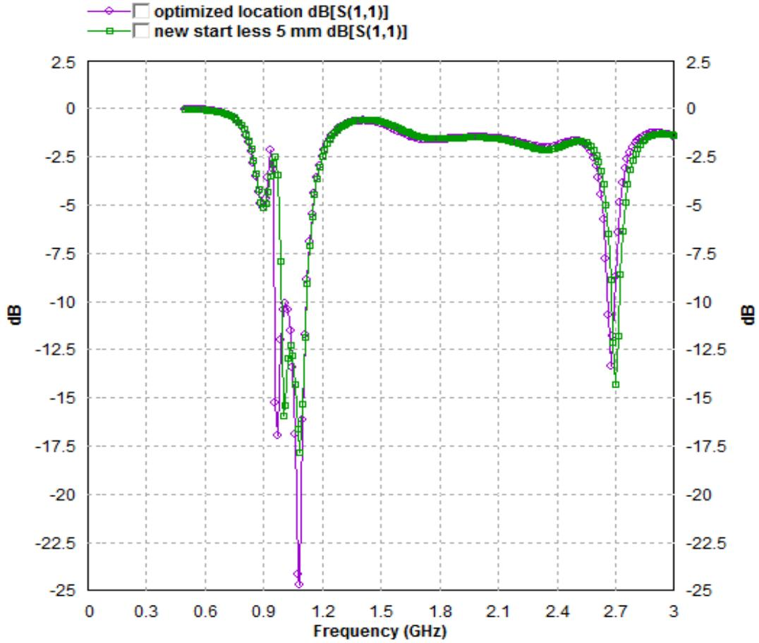
Figure 7. Return loss graph of reduced ground plane.
