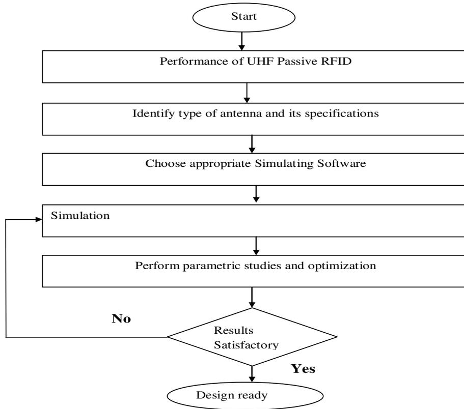
Figure 3. Flow chart on the simulation of the proposed antenna.
