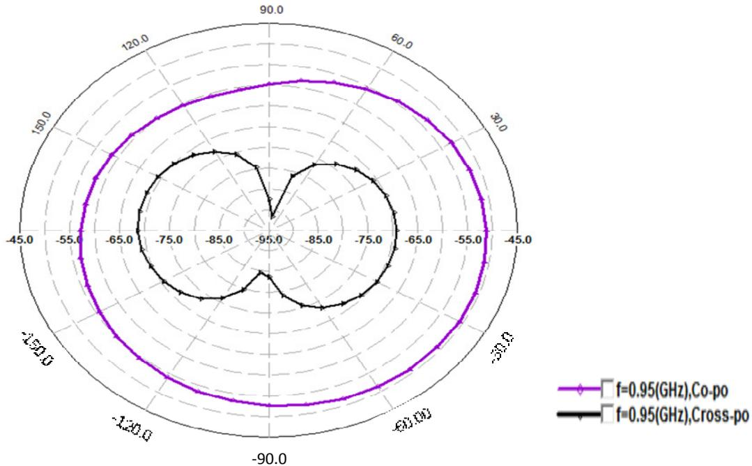
Figure 6b. Azimuth pattern gain display at 90°.
