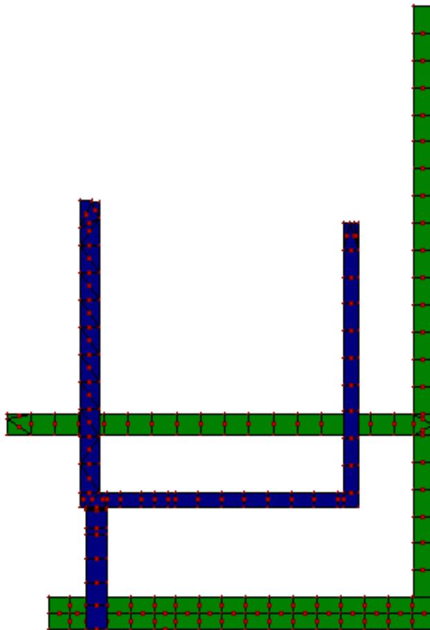
**Figure 9.** Current distribution of the proposed antenna.
