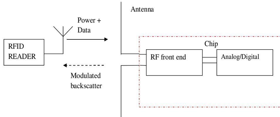
**Figure 1.** RFID system operation; Source: (Yu et al., 2006).
