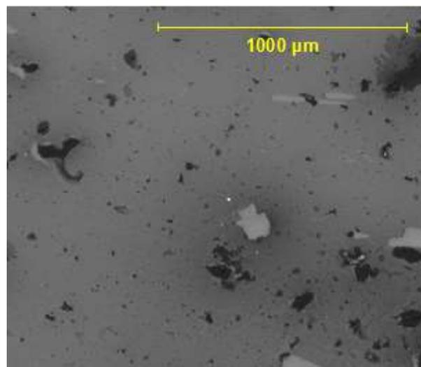
**Figure 7.** SEM image of P3HT:PCBM unannealed.
