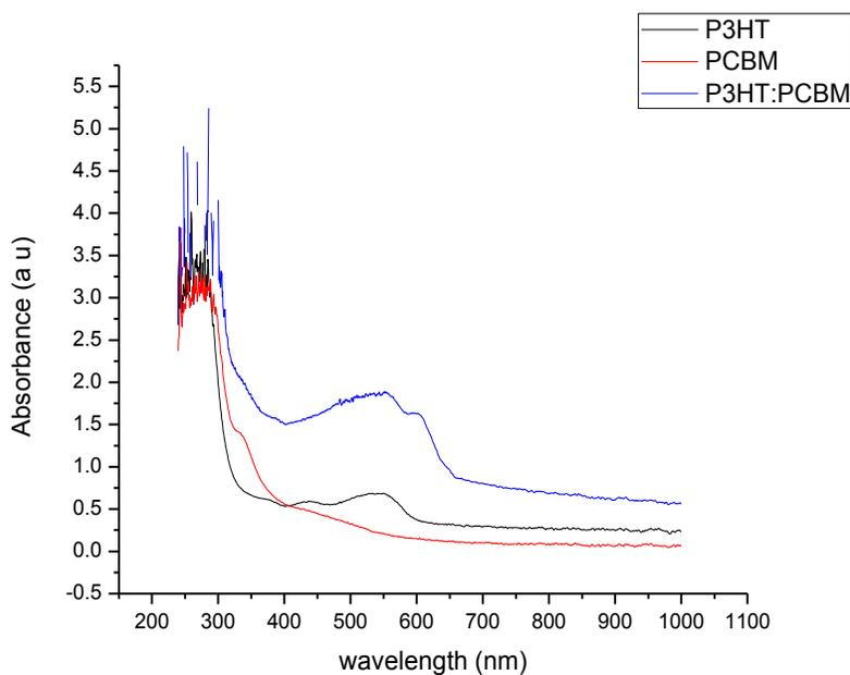
**Figure 16.** Absorbance of P3HT, PC<sub>61</sub>BM, and P3HT:PC<sub>61</sub>BM thin films at 70°C graph.
