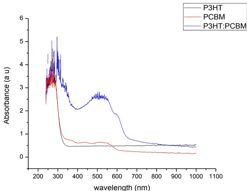
**Figure 17.** Absorbance of P3HT, PC<sub>61</sub>BM, and P3HT:PC<sub>61</sub>BM thin films at 80°C graph.
