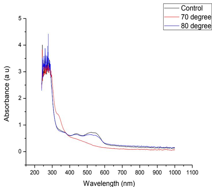
Figure 14. Plot of absorbance vs. wavelength graph of PC<sub>61</sub>BM.
