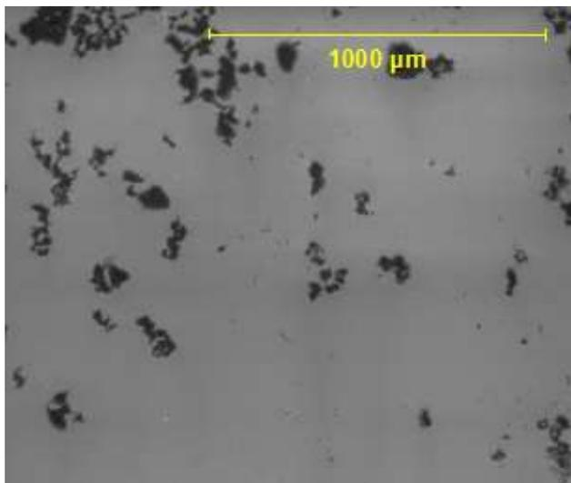
**Figure 1.** SEM image of P3HT unannealed (control).
