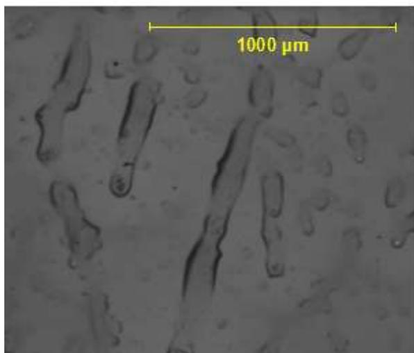
**Figure 5.** SEM image of PC<sub>61</sub>BM at 70°C.
