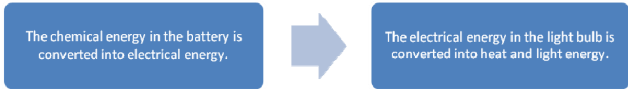
Figure 1. Energy conversion in a simple electrical circuit.
