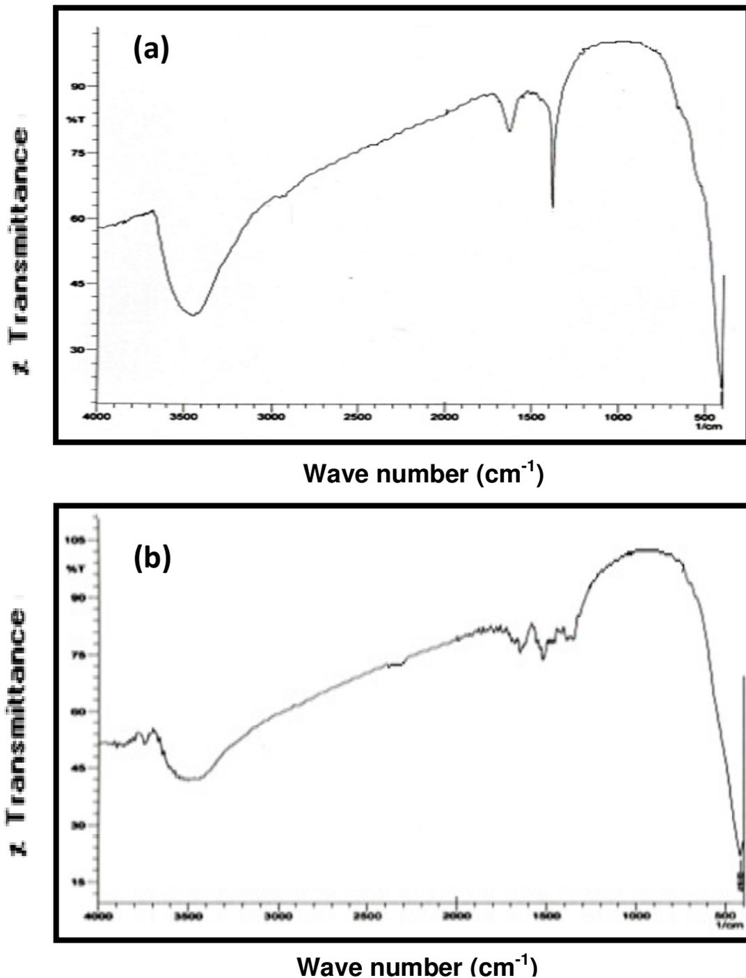
Figure 2. The IR spectra. (a) Precursor and (b) calcined powder.
