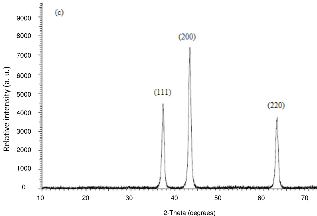
**Figure 1.** XRD patterns of the precursor (a), and calcined powders at 300 (b), and 400 °C (c).
