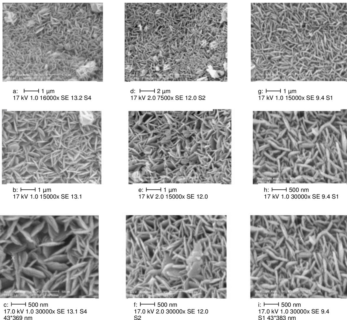
**Figure 3.** The SEM image of (a, b, c) precursor and calcined powder at (d, e, f) 300, and (g, h, i) 400°C.
