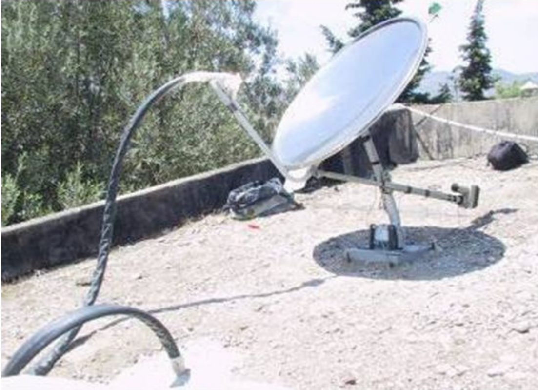
Figure 10. One example of the heliostats solar concentrator and light transmission through optical fibers (Kandilli et al., 2008: 23).
