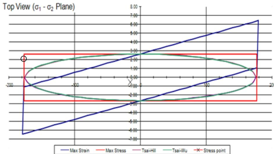
**Figure 4.** Failure criterion graphics in KSI unit.
