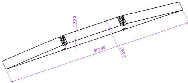
Figure 1. Dimension of beam with 3 sections connected.
