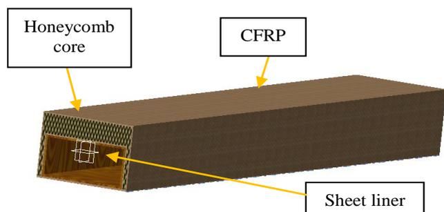
**Figure 3.** The location of honeycomb (core structure) on the mid-section.
