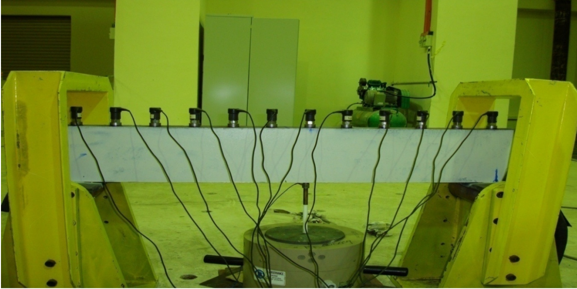
Figure 2. Test setup for the solid steel beam.
