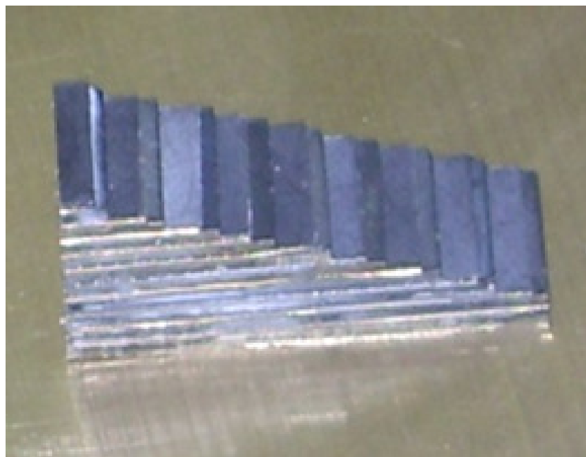
Figure 1. The tunable NRIM sample. (a) Structure of the tunable NRIM sample and (b) photo of the tunable NRIM sample.
