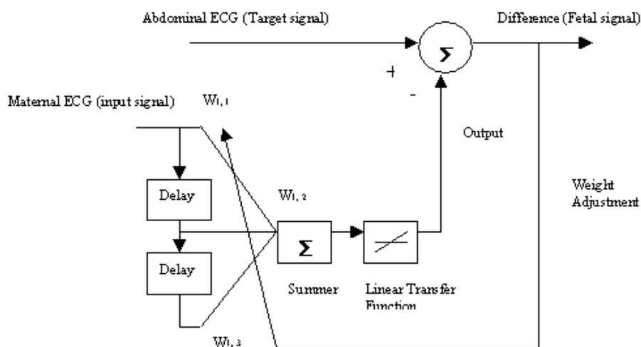
**Figure 2.** Adaptive linear neural network filter architecture.
