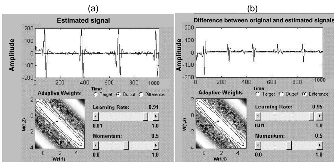
Figure 4. (a) Estimated signal and (b) difference signal (fetal ECG) when learning rate was high.
