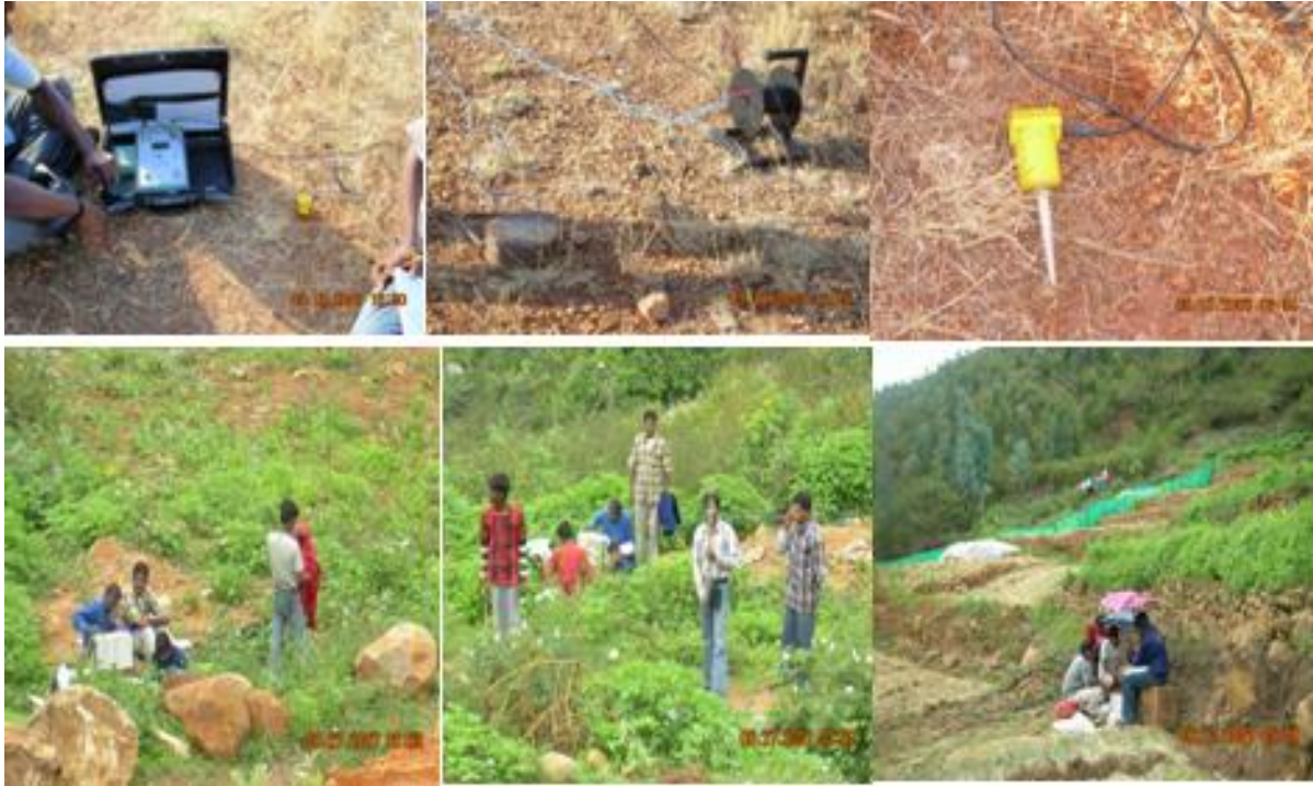
Figure 2. Seismic refraction and 2D Electrical Resistivity Imaging (ERI) data collection in the Ooty landslide area.
