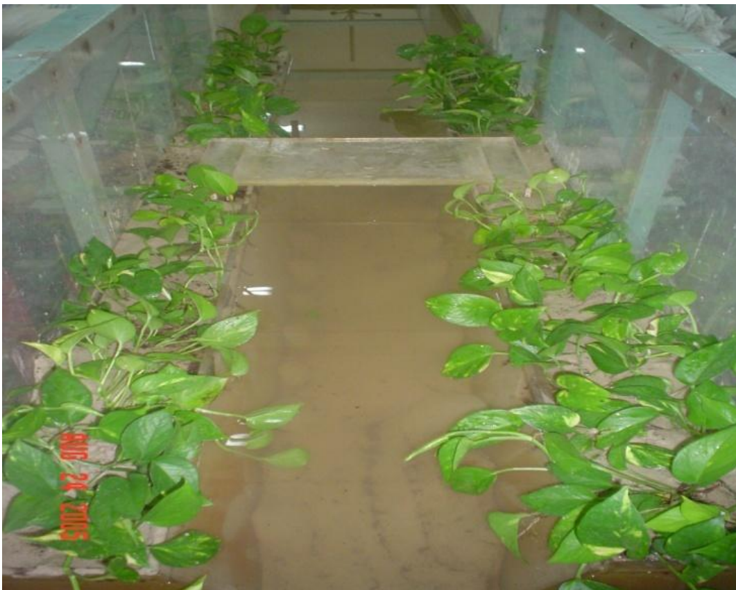
Figure 7. Integral bridge model with E. Aureum planted along floodplains.
