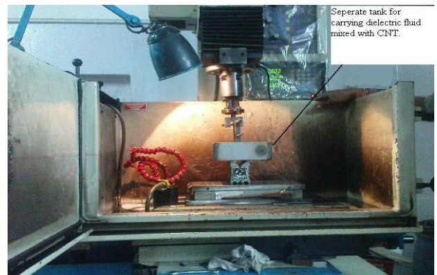
Figure 3. EDM set up using MWCNT.
