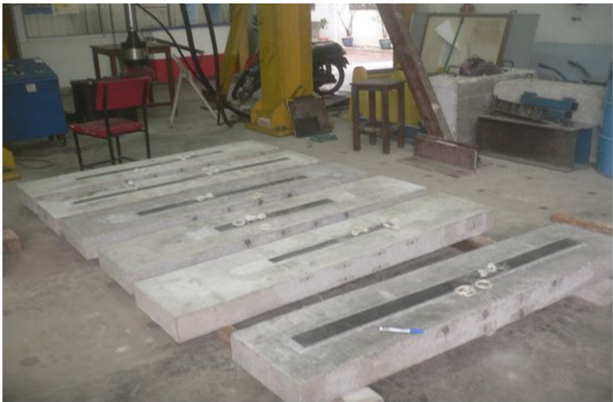
Picture 1. RC one-way slab strengthened by different lengths and width of CFRP.
