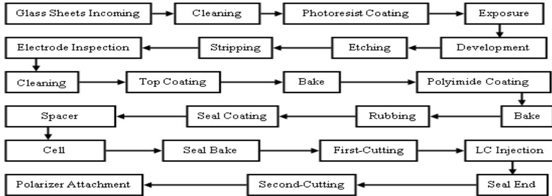
Figure 1. Flow-chart of STN- LCD manufacturing process.
