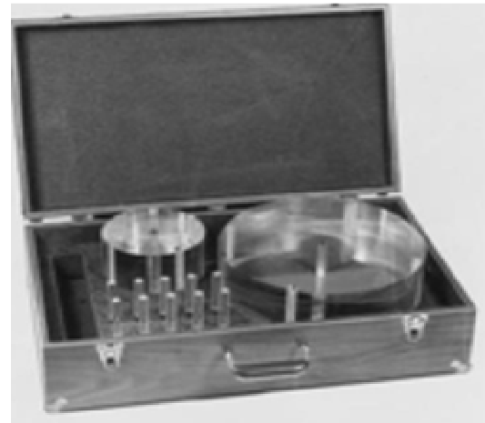
Figure 2. Typical phantom used for determination of CTDI.
