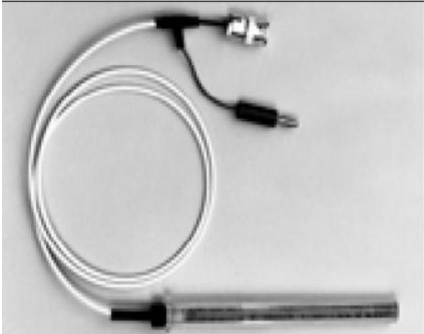
Figure 3. 10 cm ionization chamber used with the phantom for determination of CTDI.
