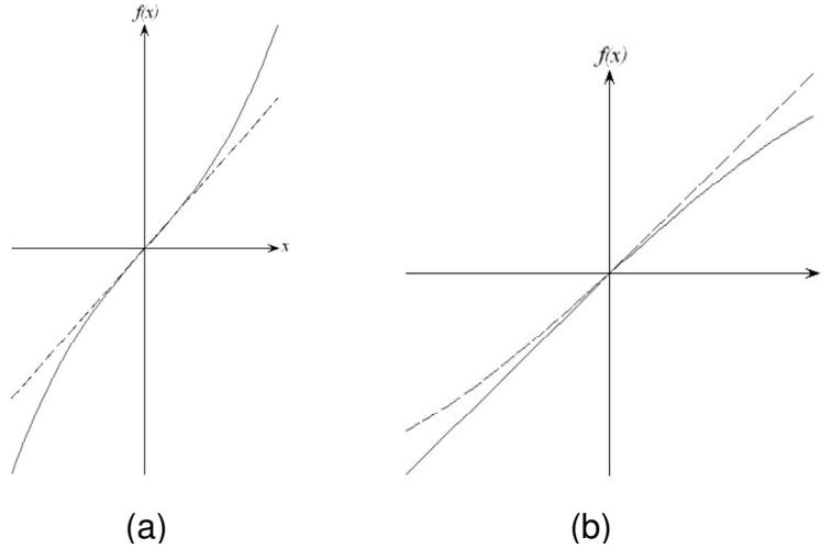
**Figure 2.** (a) Hard spring stiffness nonlinear behavior. (b) Soft spring stiffness nonlinear behavior.
