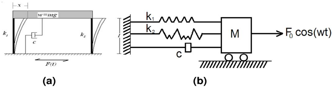
**Figure 1.** (a) Schematic view of a structure under harmonic load. (b) The dynamic model of a structure under harmonic load.
