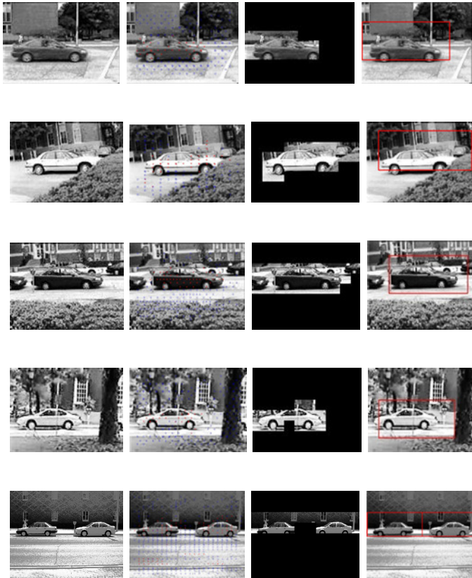
Figure 2. Detection results in UIUC database. The first column is original images, the second column is results of local feature response, the third column is detection results using our proposed method, and the last column is final detection results based on simple fusion method.
