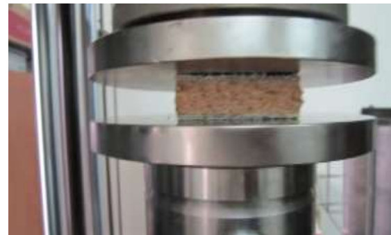
Figure 2. Specimen sandwich in the compression test.
