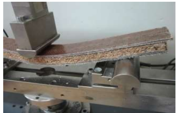
Figure 8. Bending tests three items, after fracture.
